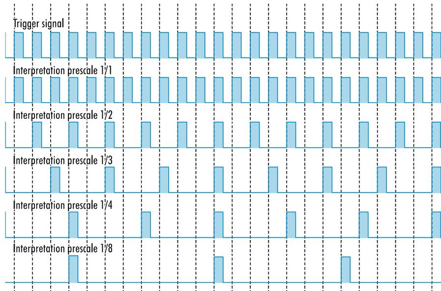
Fig. 5-46: Prescale values and their result on trigger signal
