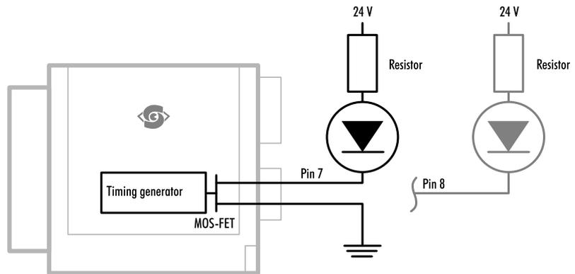
Fig. 5-37: Attach LED lights to camera outputs
