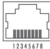
Fig. 3-1: RJ45 socket connector
