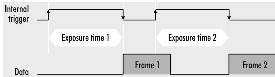
Fig. 5-28: Mode 0 - Free running with programmable exposure time
