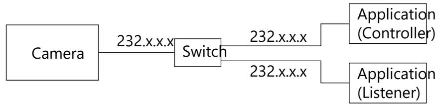
Fig. 3-4: Camera casting to multiple receivers (multicast)
