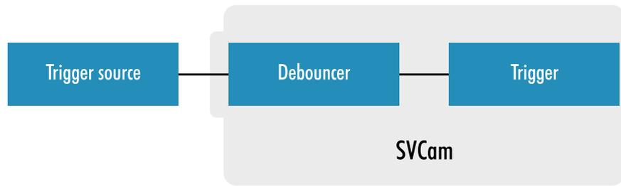
Fig. 5-44: Debouncer between the trigger source and trigger
