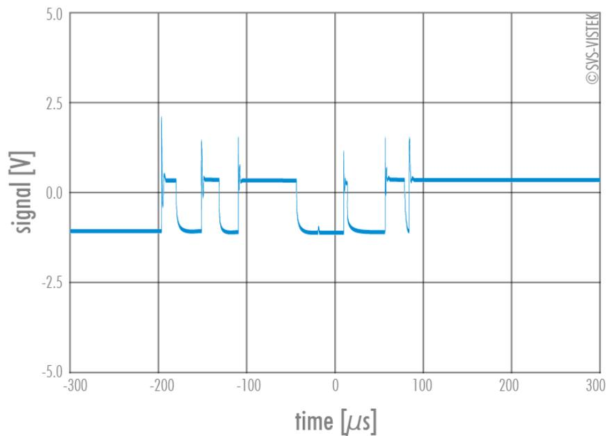
Fig. 5-43: Bounces or glitches caused by a switch
