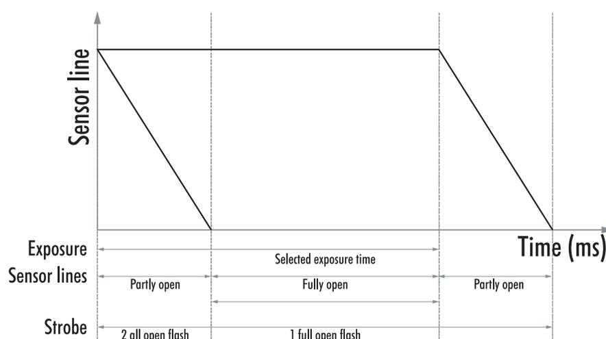
Fig. 5-18: Flash control with rolling shutter
