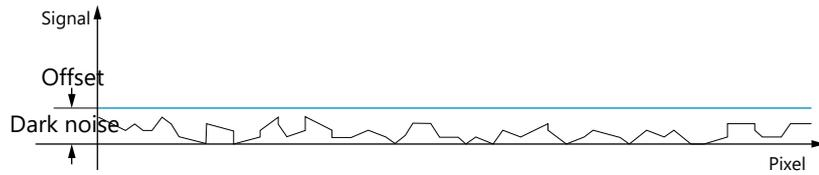
Fig. 5-2: Dark noise cut off by the offset
