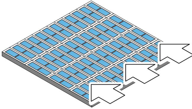
Fig. 5-7: Vertical binning
