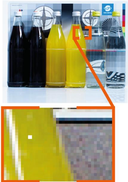
Fig. 5-23: Illustration of a defect pixel
