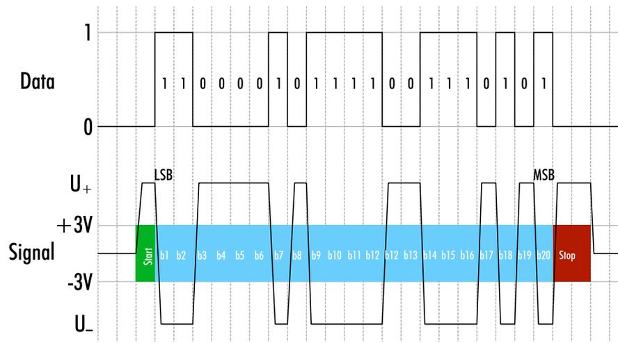
Fig. 5-41: UART encoding of a data stream
