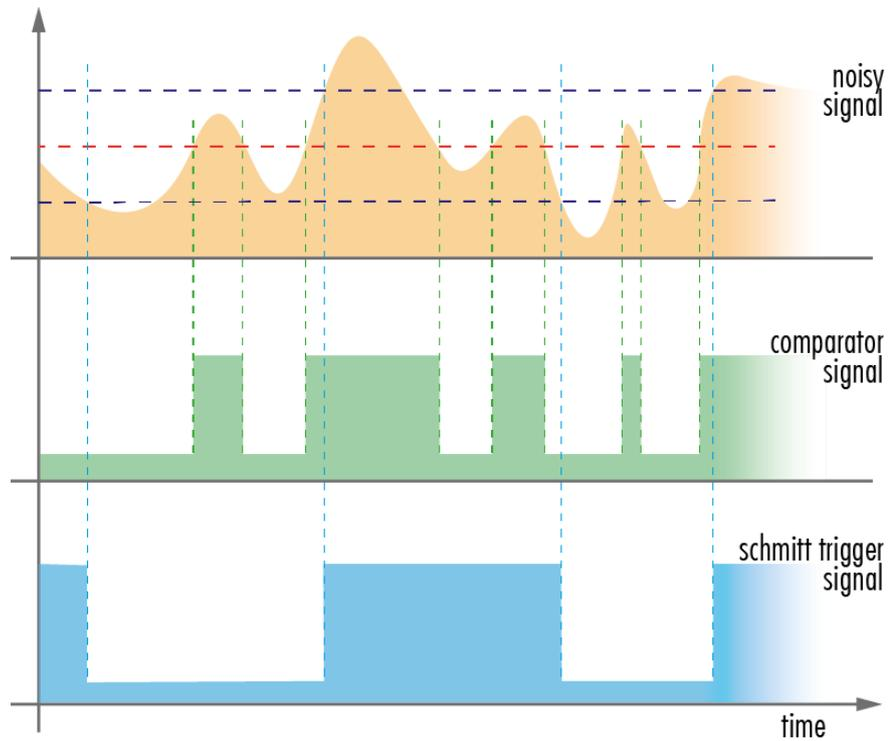
Fig. 5-42: Schmitt trigger noise suppression
