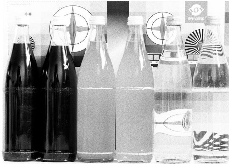
Fig. 5-1: Noise caused by too much gain
