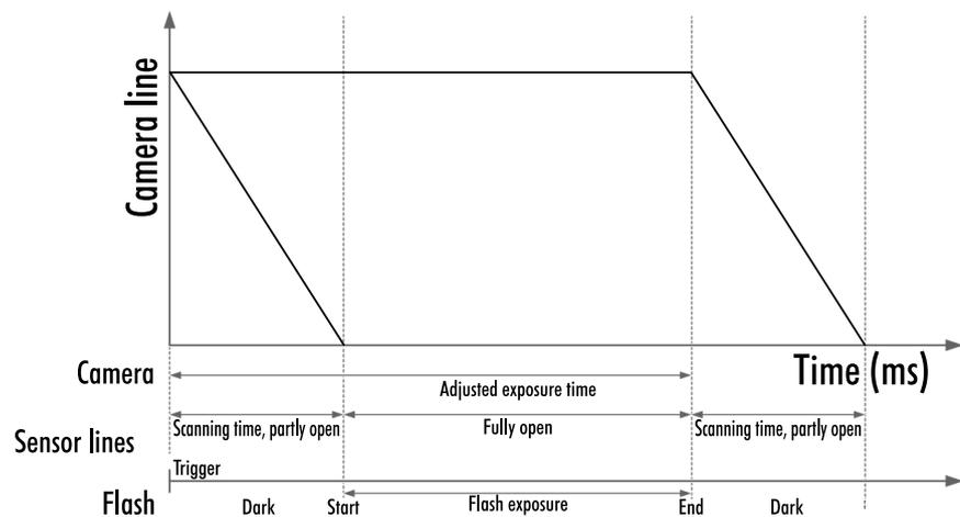
Fig. 5-19: Rolling shutter lines light sensitivity versus time
