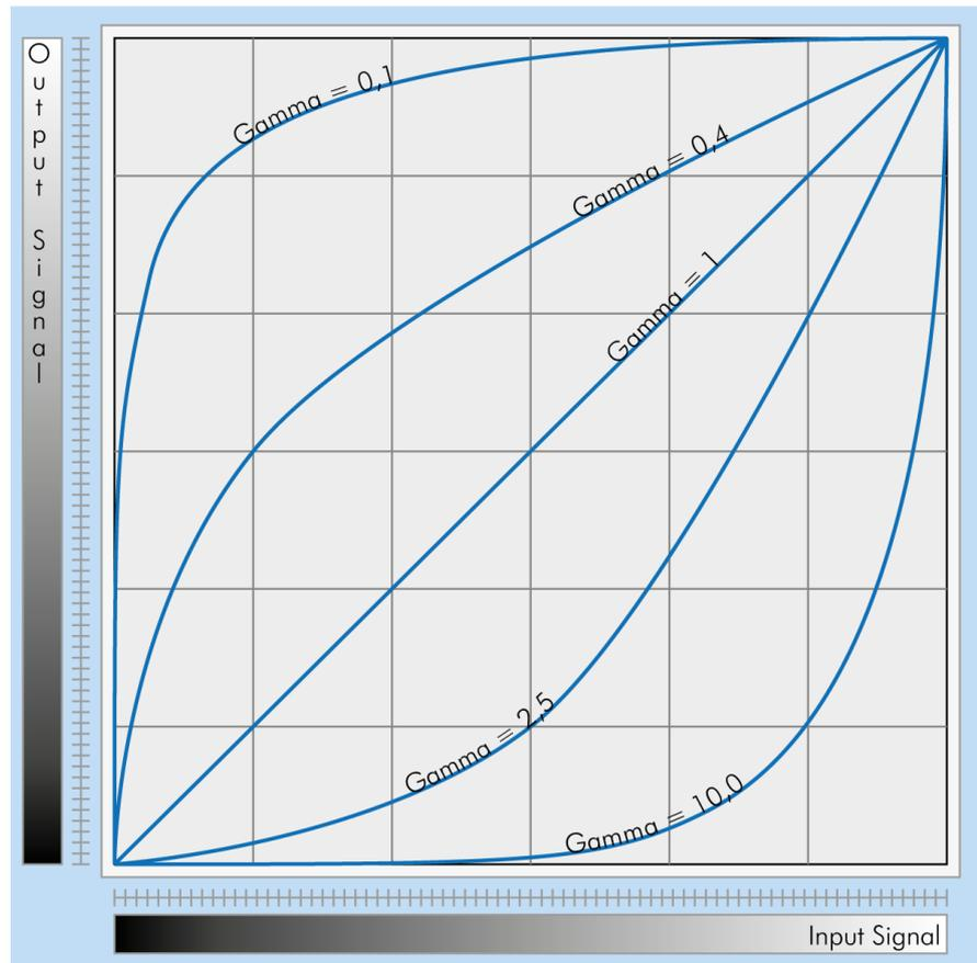
Fig. 5-26: Several gamma curves comparable to a LUT
