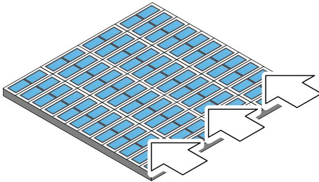
Fig. 5-8: Horizontal binning
