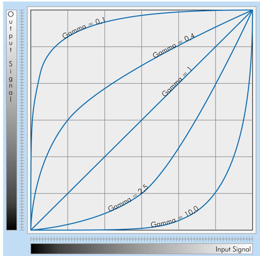
Fig. 5-25: Several gamma curves comparable to a LUT
