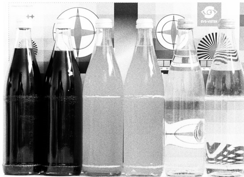
Fig.: 6-1: Noise caused by too much gain
