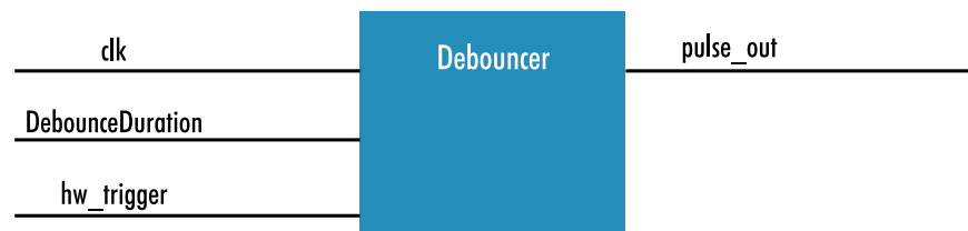
Fig. 5-52: The debouncer module
