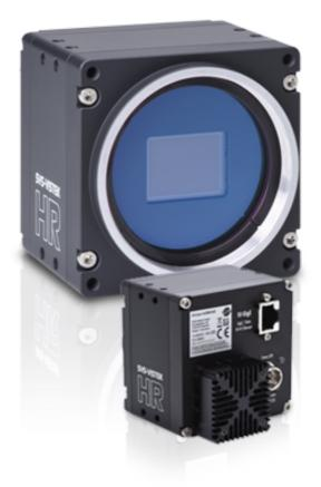
The HR 10 GigE series with its high-end high-resolution CCD and CMOS sensors permits making full use of the sensor bandwidth. 10 GigE delivers up to 1.1 GB/s of image data with distances up to 100m .
