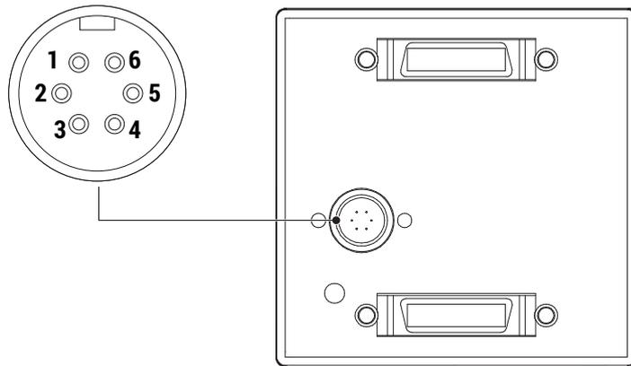
Fig.: 4-1: Power connector pinning
