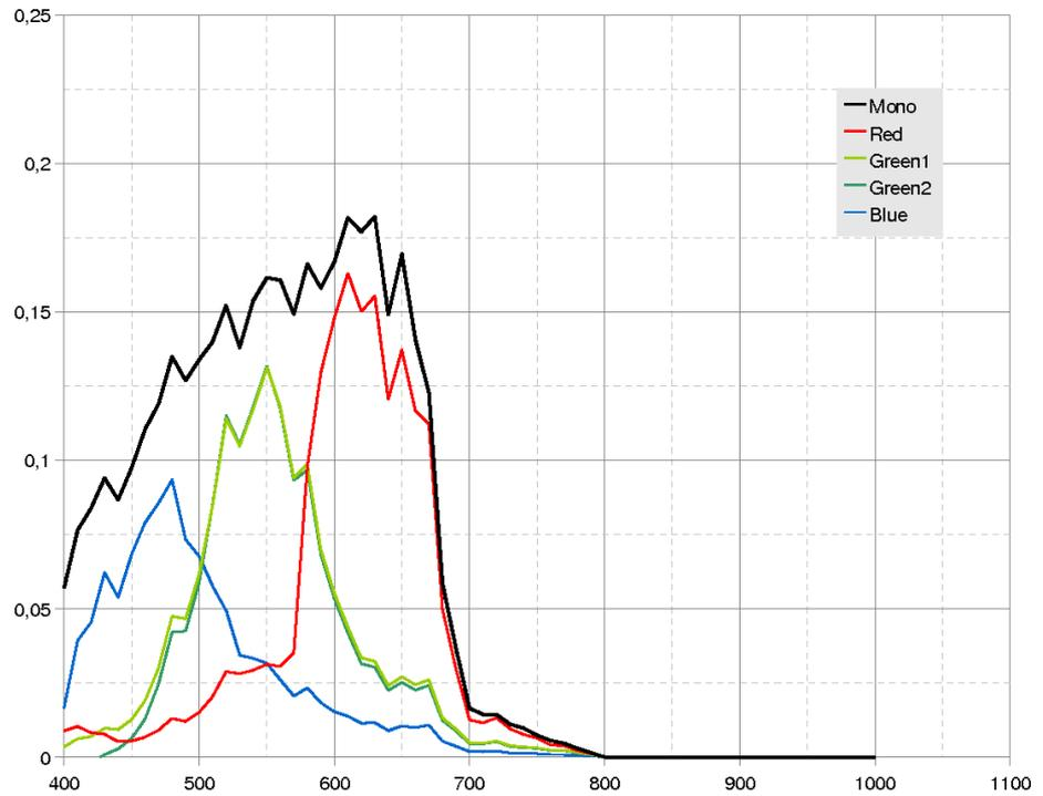
Fig.: 5-3: Quantum Efficiency mono and color with UV/IR Cut Filter
