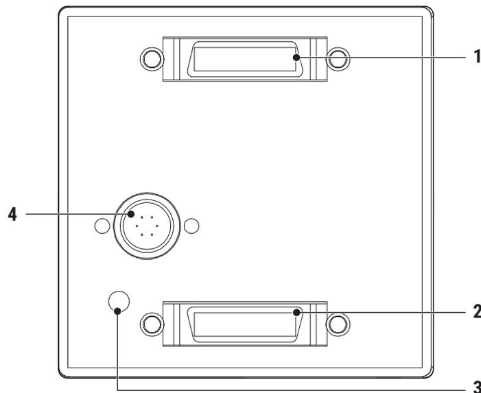
Fig.: 3-1: Interfaces of the camera EoSens® 3CL
