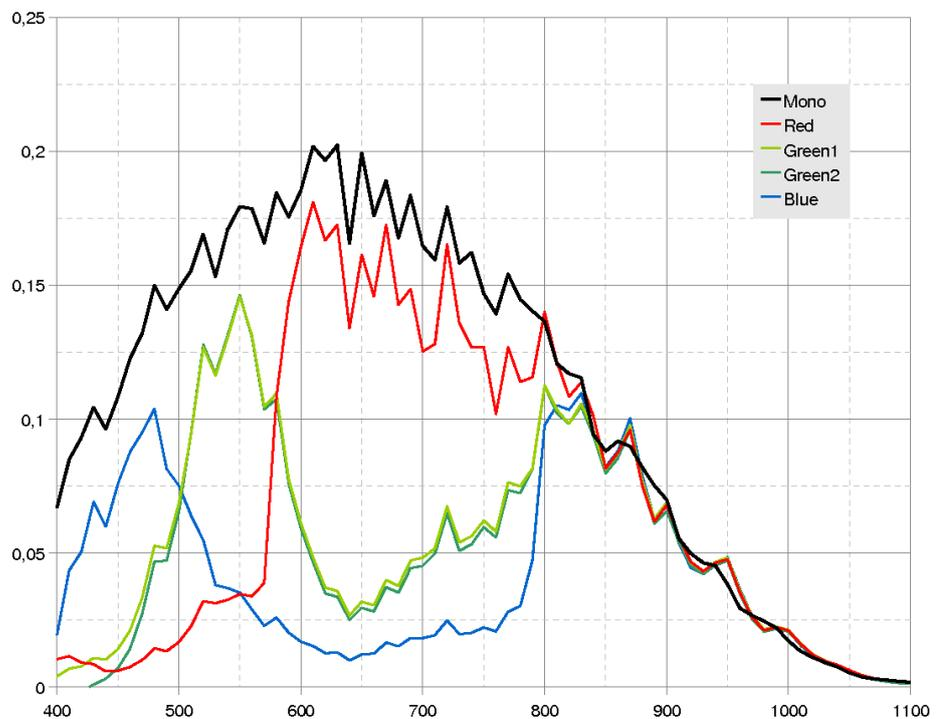
Fig.: 5-4: Quantum Efficiency mono and color without UV/IR Cut Filter
