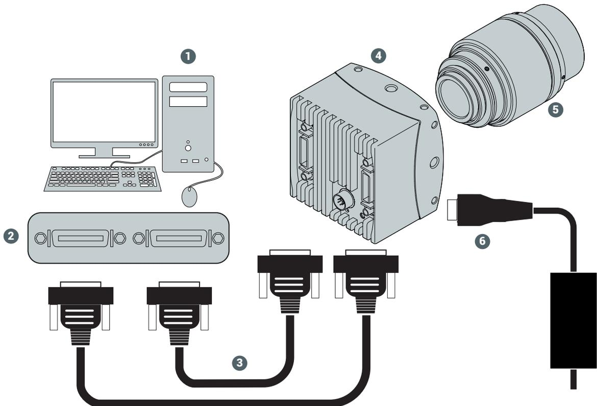
Fig.: 4-3: Connecting camera and image processing system
