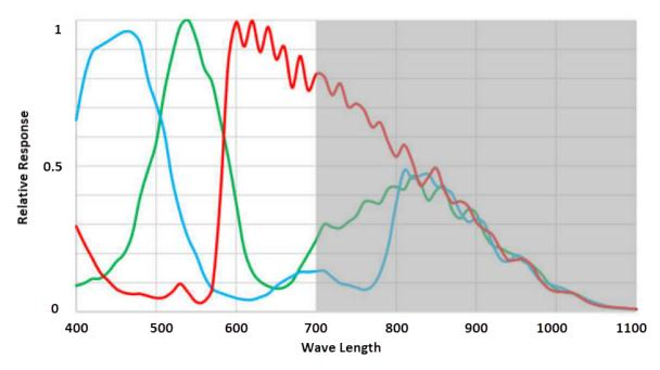
Note: The IR cut filter blocks wavelength exceeding 700nm.
