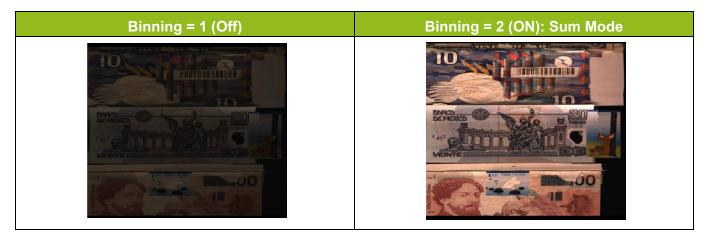
This camera supports Horizontal x2 digital binning on the FPGA.
