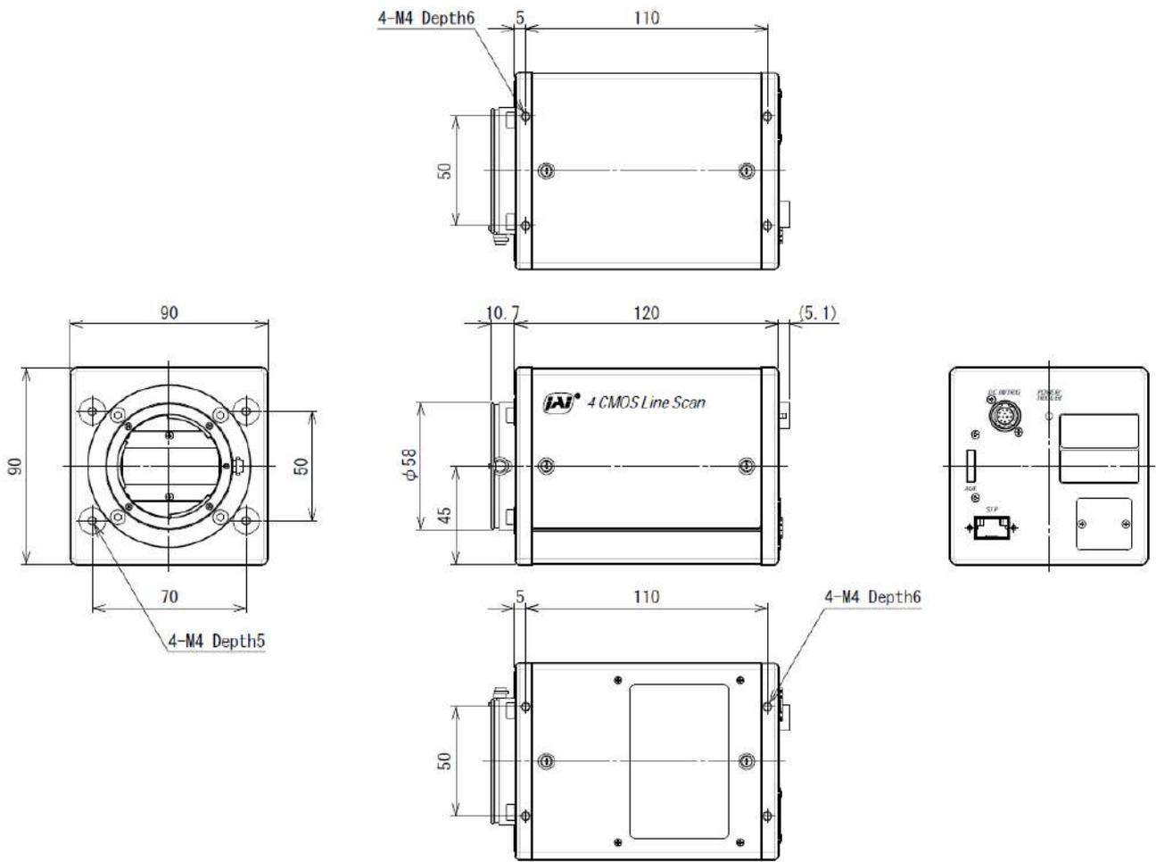
Dimensional tolerance:  $\pm 0.3\text{mm}$
