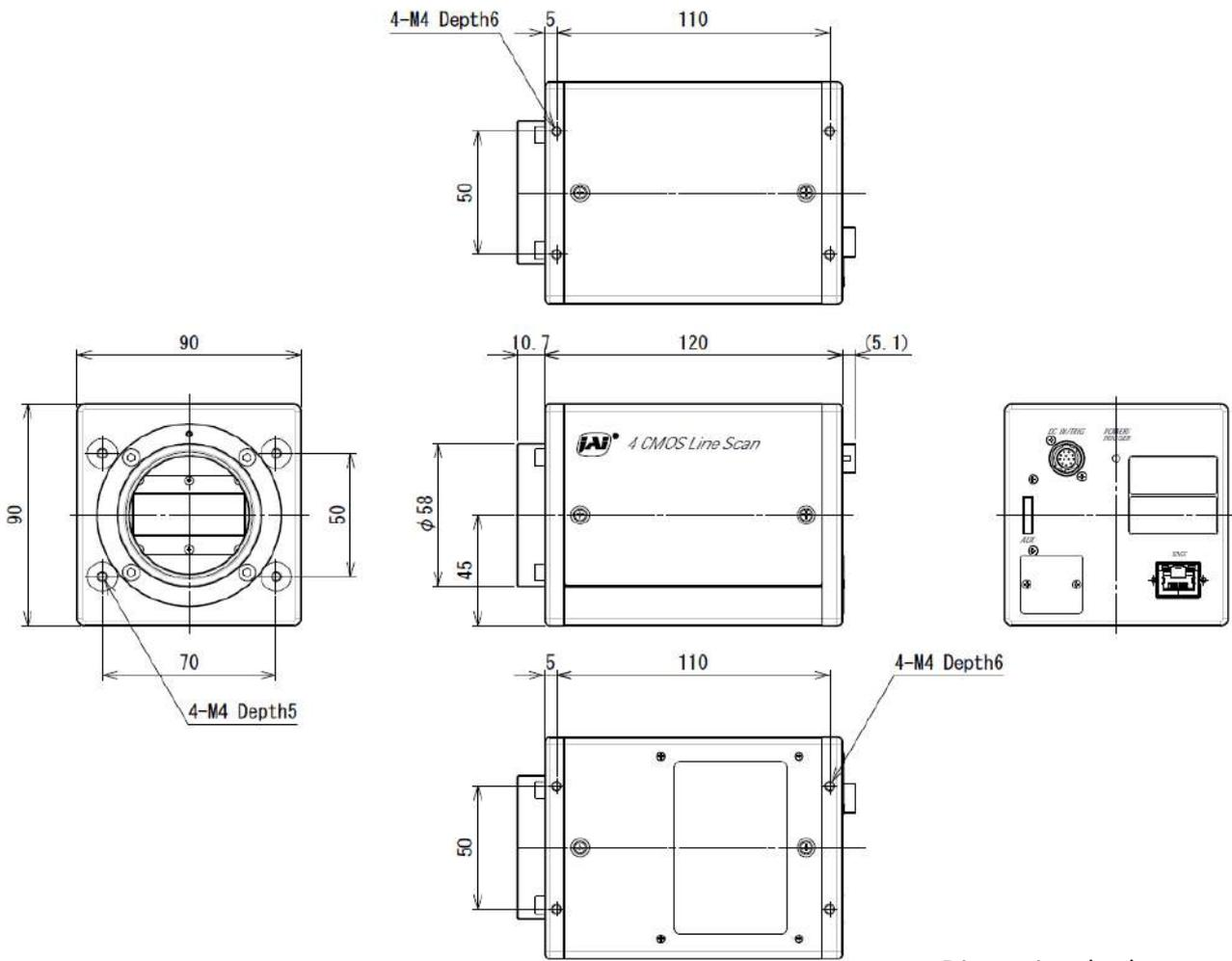
Dimensional tolerance:  $\pm 0.3\text{mm}$
