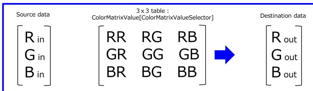
Configuration 3x3 table. Select the item you want to configure in [ColorMatrixValueSelector]. And configure the value in [ColorMatrixValue]. [ColorMatrixValue] can be set to a value from -2 to +2.
