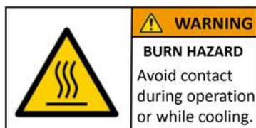
Depending on the operating environment, the surface of the camera may become very hot during operation. Do not touch the camera during operation and while it is being cooled.
