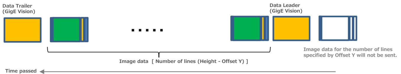
When using Frame Start Trigger, after receiving Frame Start Trigger, skip the image data of the number of lines of Offset Y and send the data of Data Leader, image data, Data Trailer.
