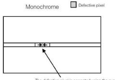
The defective pixel is corrected using the average value between the pixels to the immediate left and right.
