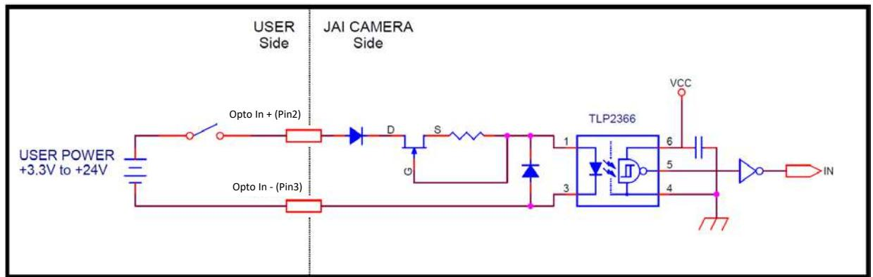
■ Recommended external output circuit diagram (reference example)
