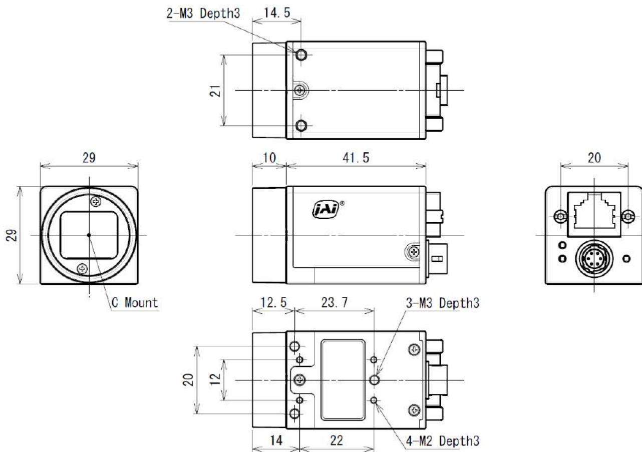
Dimensional tolerance:  $\pm 0.3\text{mm}$
