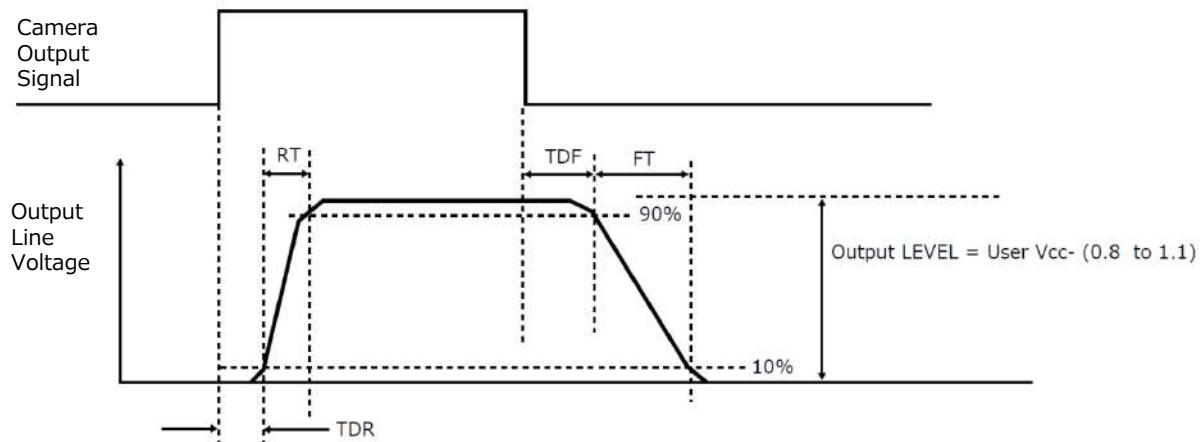
For the operating conditions of applied voltage (User Power) +12V, load resistance 10kΩ, and cable length 1m, the timing is shown in the table below.
