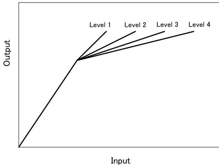
Fig.39 HDR characteristics
