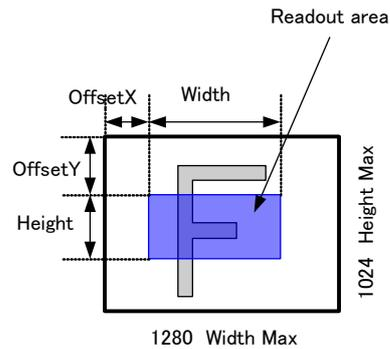
Fig.20 Setting example (Binning)
