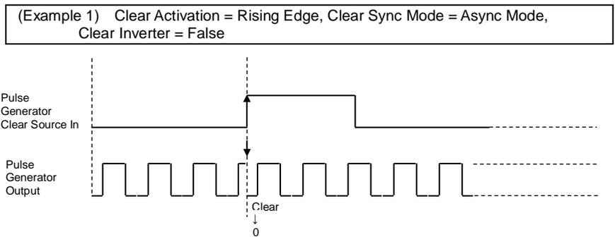
Fig.12 Counter clear in Async mode
