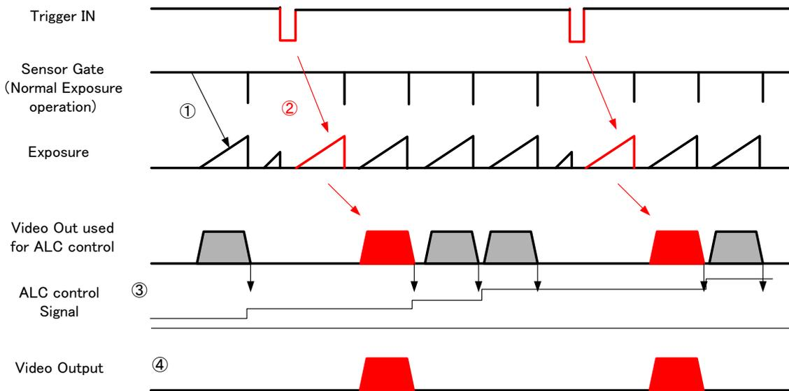
Fig.25 RCT mode timing for ALC operation (Example)
