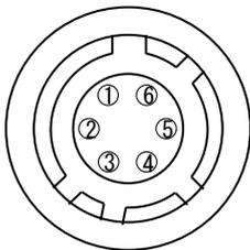
Fig.5 6-pin connector
