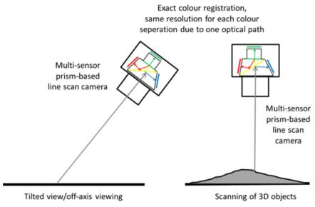
Fig. 6 - Prism-based line scan cameras in off-axis and 3D object inspection
