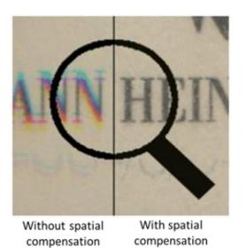
Fig. 9 - Spatial compensation in trilinear cameras (image from AIA training material)
