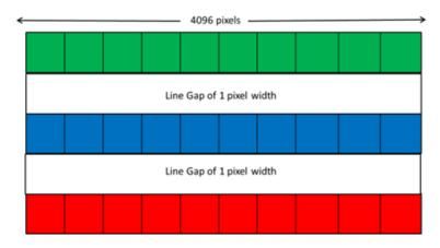
Fig. 8 - Spatial compensation in trilinear cameras (image from AIA training material)
