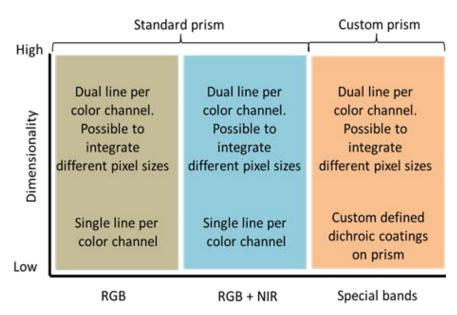
Fig. 3 - Configurations with multi-sensor prism-based line scan cameras
