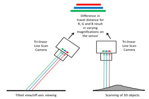
Fig. 4 - Off-axis viewing and inspecting 3D objects with trilinear line scan camera
