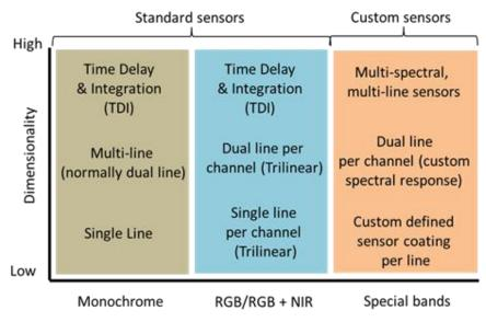
Fig. 2 - Configurations with single-sensor line scan cameras
