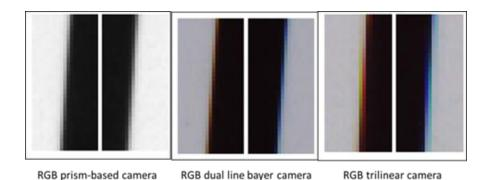
Fig. 7 - Image quality of a moving printed web using different camera technologies
