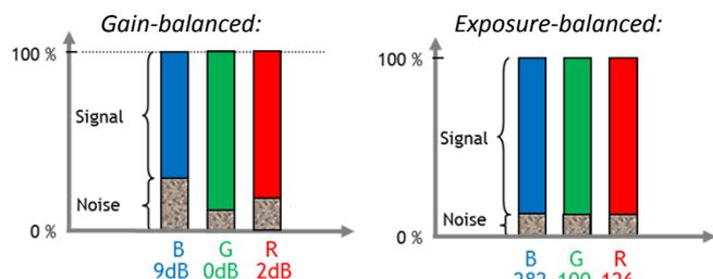
Notice for the gain-balanced system, the available signal for the higher gain channels is reduced, while exposure-balancing restores the full signal range. The combination of maximizing the signal in each channel with lowering the noise, further increases dynamic range and color fidelity.
