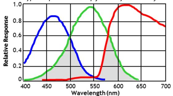
**High Dynamic Range** - In addition to reducing color precision, the overlap in the color filter response also results in part of each pixel's well capacity filling with photons resulting from the crosstalk, thus decreasing the available well capacity. Precision responses from the dichroic coatings enable each channel to efficiently use the full well capacity of the pixel, allowing the maximum possible dynamic range.
