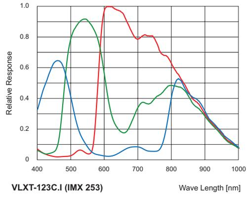
Figure 4: Spectral sensitivities for Baumer cameras with 12.3 MP sensor.
