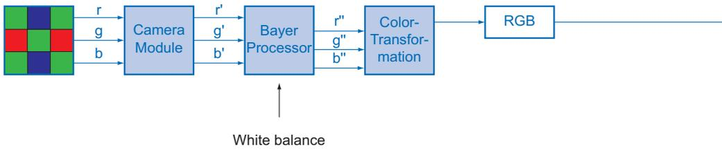
Figure 5: Color processing modules of color cameras.
