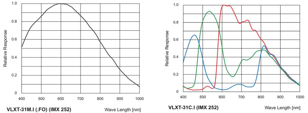
Figure 1: Spectral sensitivities for Baumer cameras with 3.1 MP sensor.
