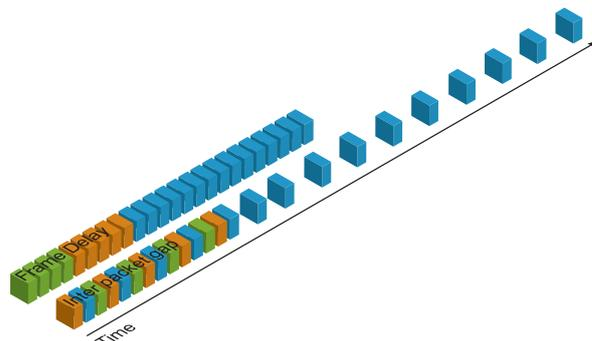
For the above mentioned example, the employment of the transmission delay feature results in a time saving – compared to the approach of using the inter packet gap – of approx. 45% (applied to the transmission of all three images).
