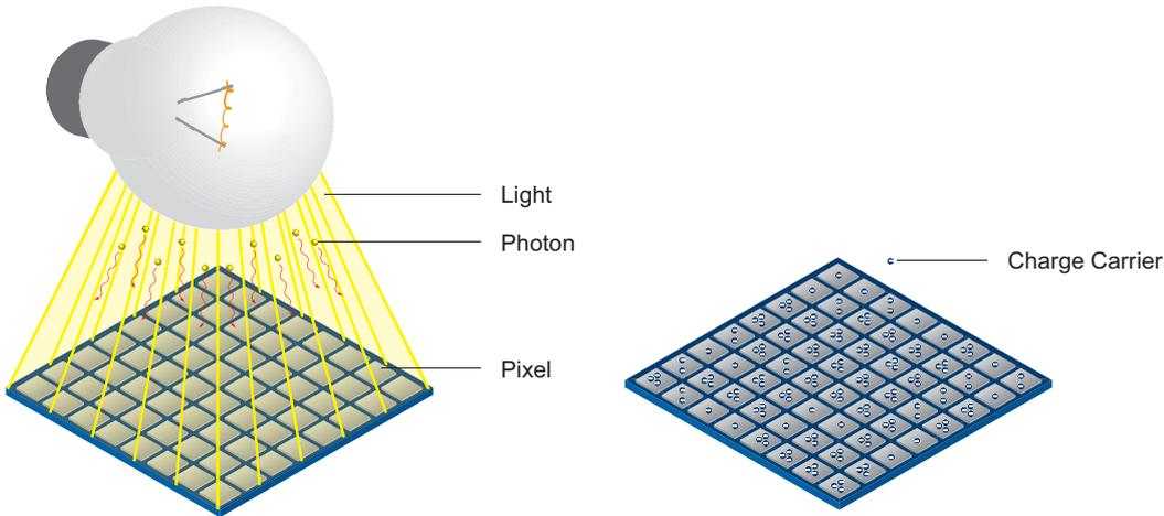
The signal strength is influenced by the incoming amount of photons. It can be increased by increasing the exposure time ( $t_{\text{exposure}}$ ).
