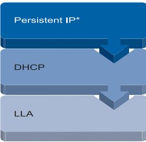
▲ Connection pathway for Baumer Gigabit Ethernet cameras:
