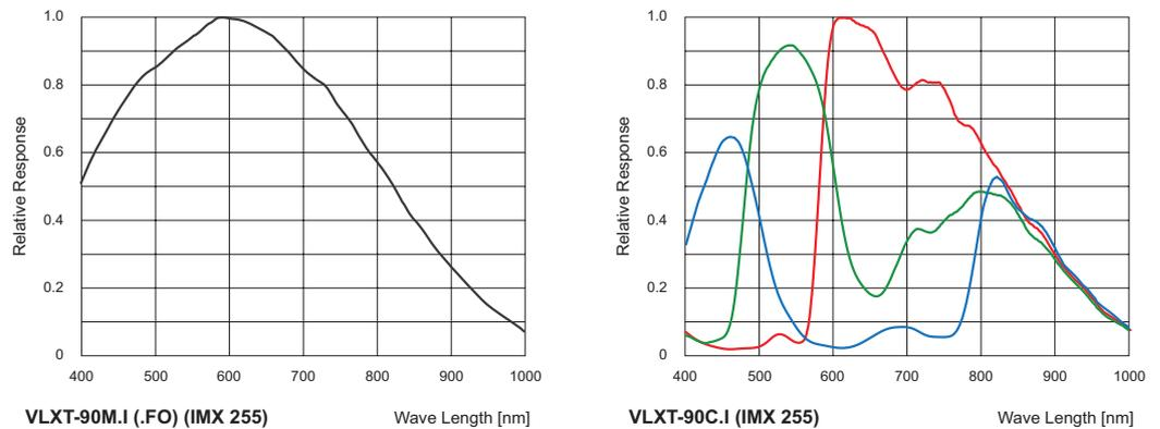
Figure 3: Spectral sensitivities for Baumer cameras with 9.0 MP sensor.
