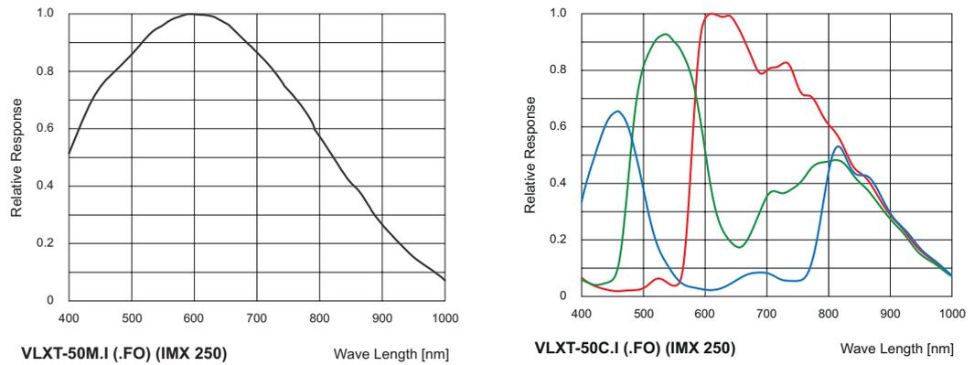
Figure 2: Spectral sensitivities for Baumer cameras with 5.0 MP sensor.
