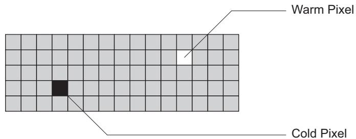
Charge quantity of "hot" and "cold" pixels compared with "normal" pixels:
