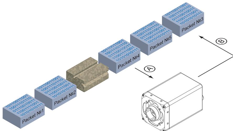
In our example packet no. 3 is lost. This fault is detected on packet no. 4, and the resend request triggered. Then the camera sends packet no. 5, followed by resending packet no. 3.
