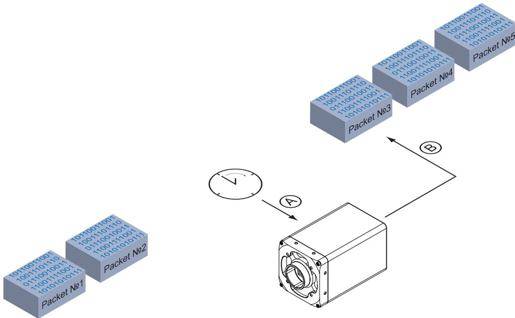
In our example, packets from no. 3 to no. 5 are lost. This fault is detected after the pre-defined time has elapsed and the resend request (A) is triggered. The camera then re-sends packets no. 3 to no. 5 (B) to complete the image transfer.
