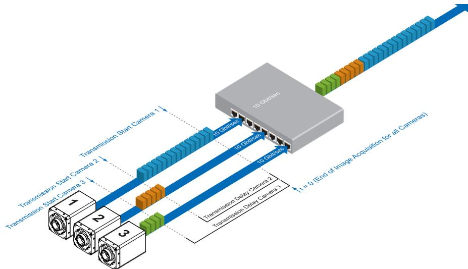
Due to process-related circumstances, the image acquisitions of all cameras end at the same time. Now the cameras are not trying to transmit their images simultaneously, but – according to the specified transmission delays – subsequently. Thereby the first camera starts the transmission immediately – with a transmission delay "0".
