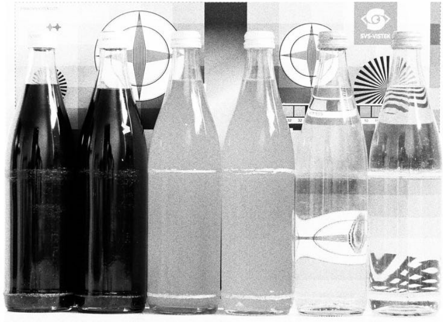
Fig. 5-1: Noise caused by too much gain
