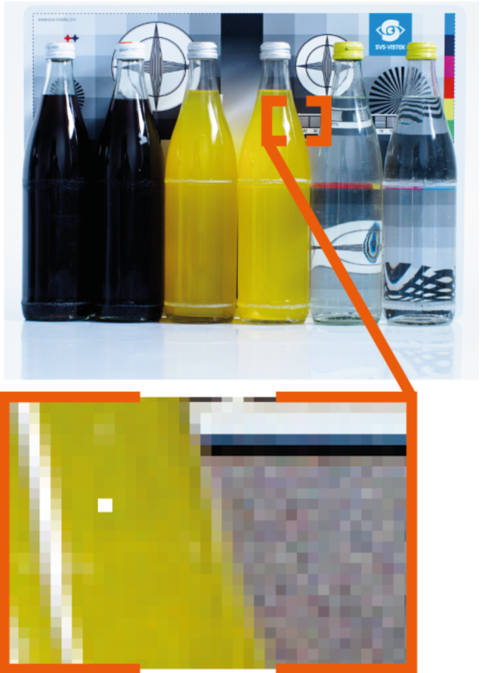
Fig. 5-22: Illustration of a defect pixel
