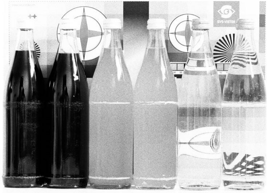
Fig. 5-1: Noise caused by too much gain
