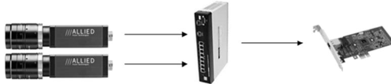
Figure 24: Multi camera network configuration using a switch and single Ethernet port
