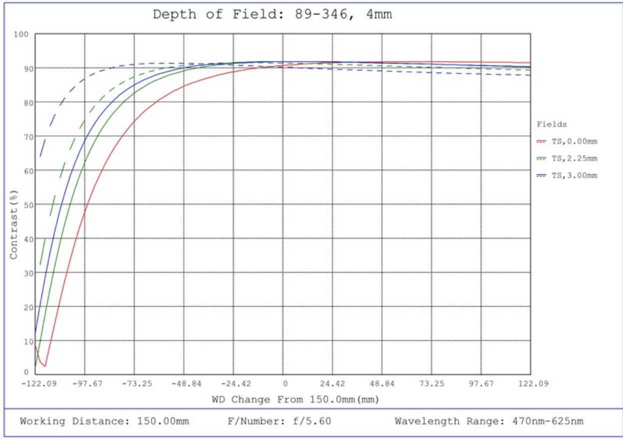
#89-346, 4mm FL f/5.6, Blue Series M12 Lens, Depth of Field Plot, 150mm Working Distance, f5.6
