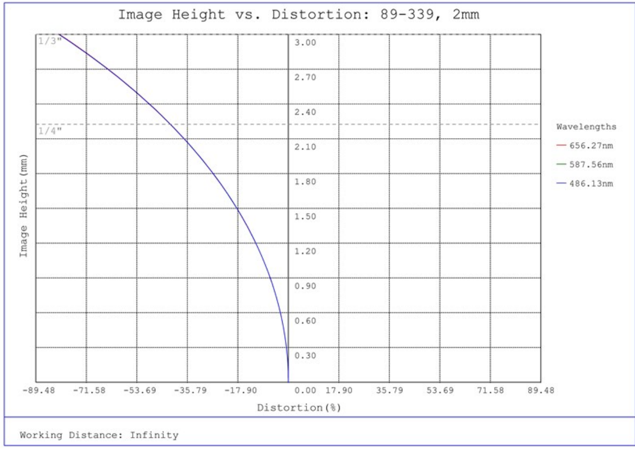
#89-339, 2mm FL f/8, Blue Series M12 Lens, Distortion Plot
