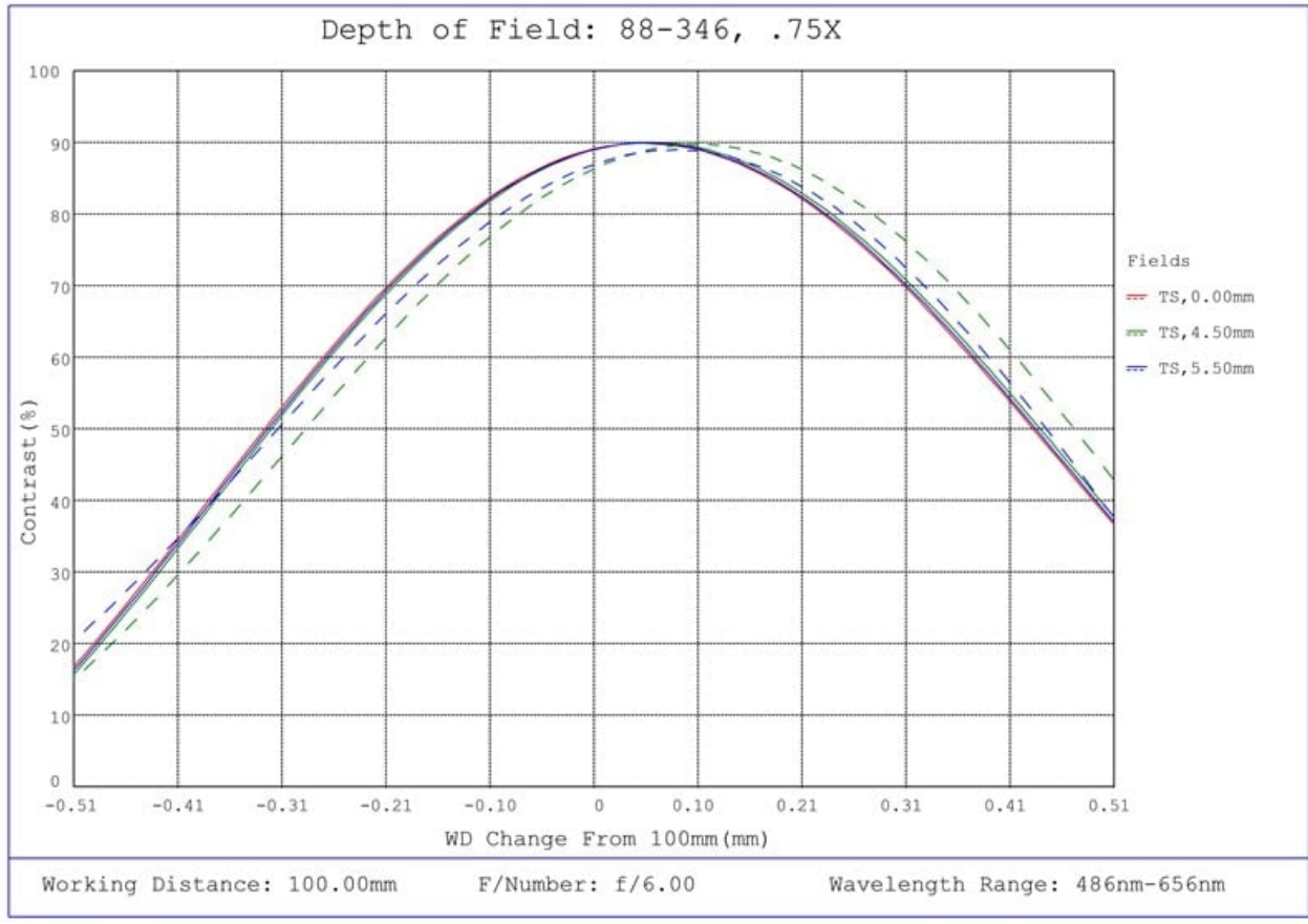
#88-346, 0.75X In-Line Illumination SilverTL™ Telecentric Lens, Depth of Field Plot, 100mm Working Distance, f6
