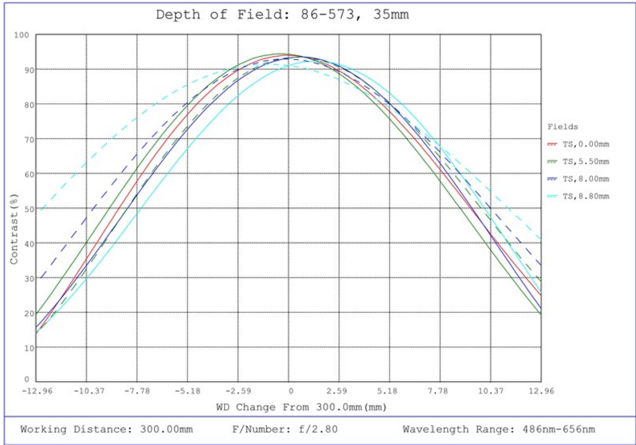
#86-573, 35mm Focal Length, HP Series Fixed Focal Length Lens, Depth of Field Plot, 300mm Working Distance, f2.8
