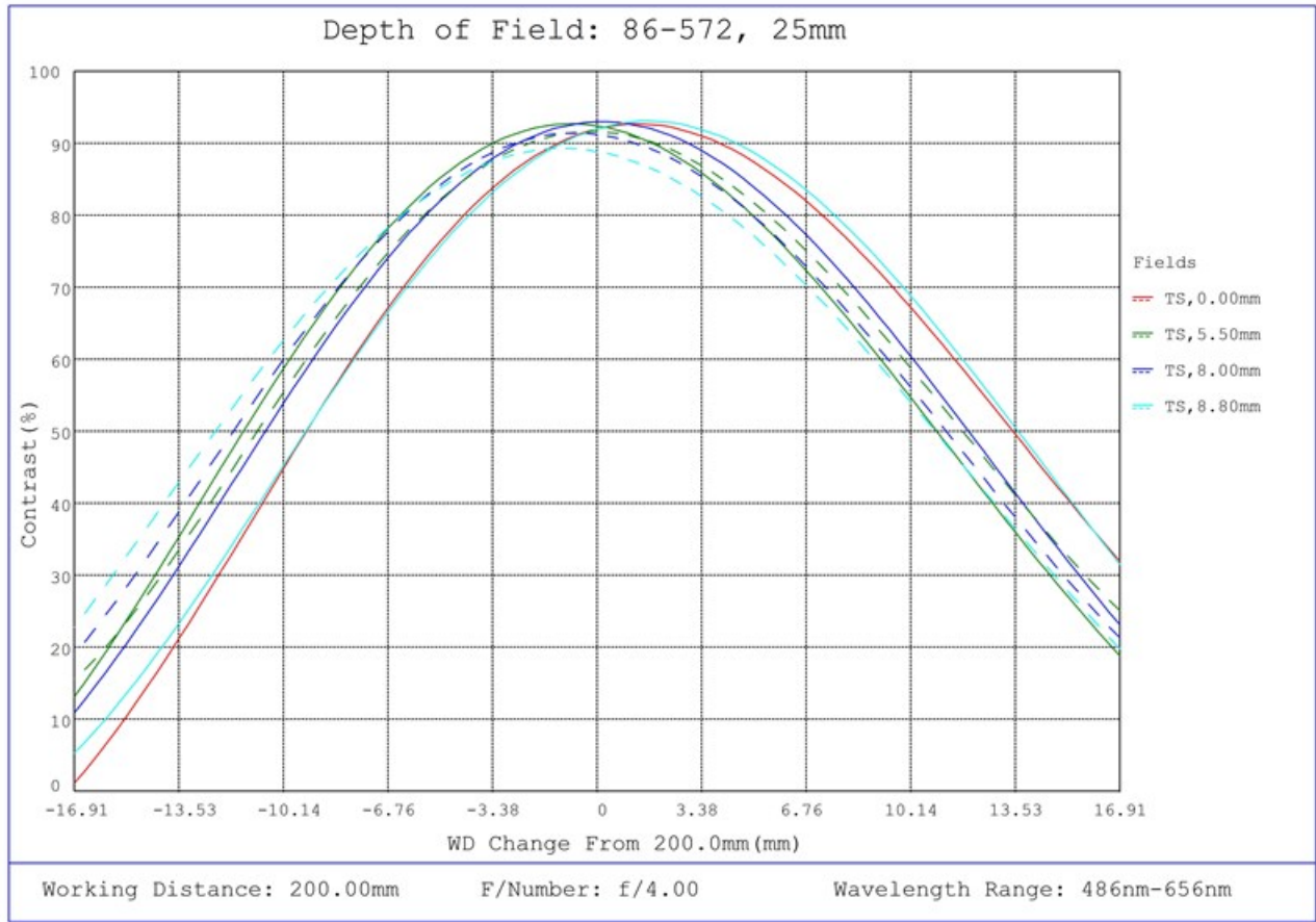
#86-572, 25mm Focal Length, HP Series Fixed Focal Length Lens, Depth of Field Plot, 200mm Working Distance, f4
