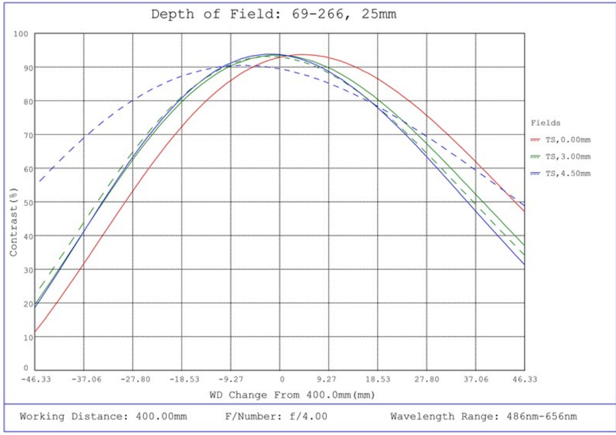
#69-266, 25mm FL f/4, Blue Series M12 Lens, Depth of Field Plot, 400mm Working Distance, f4
