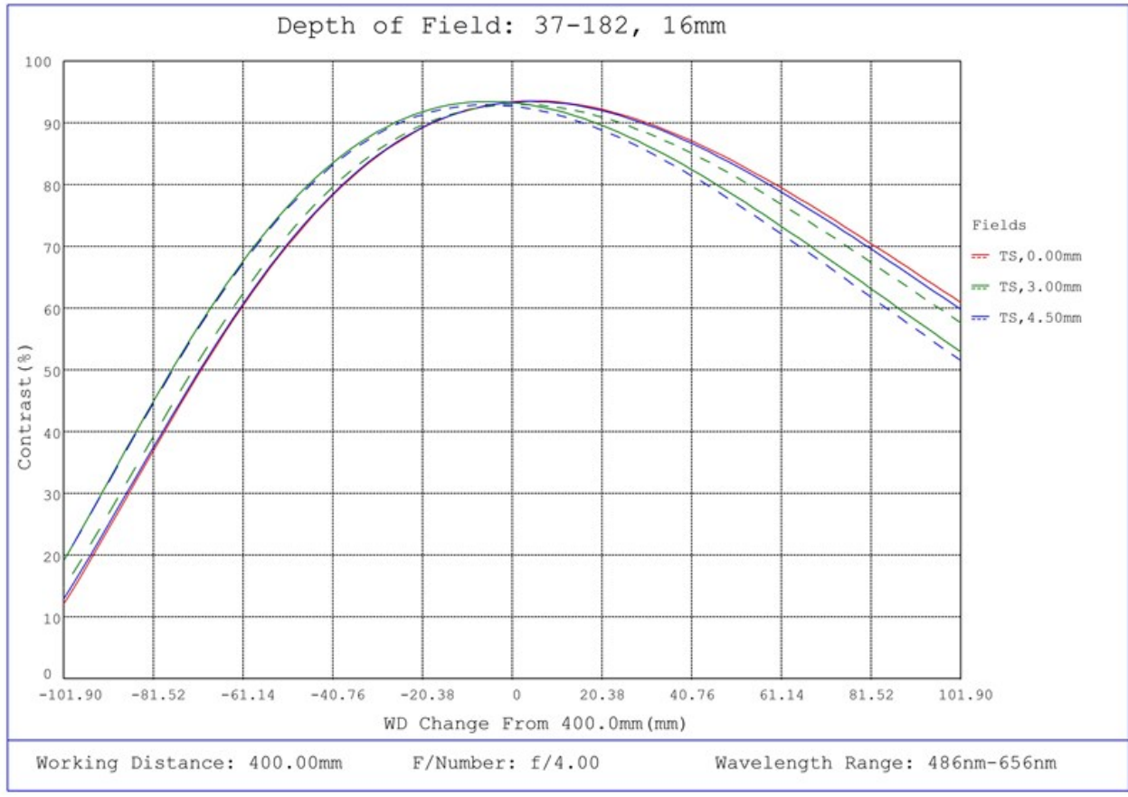
#37-182, 16mm FL f/4.0 Blue Series M12 Lens, Depth of Field Plot, 400mm Working Distance, f4
