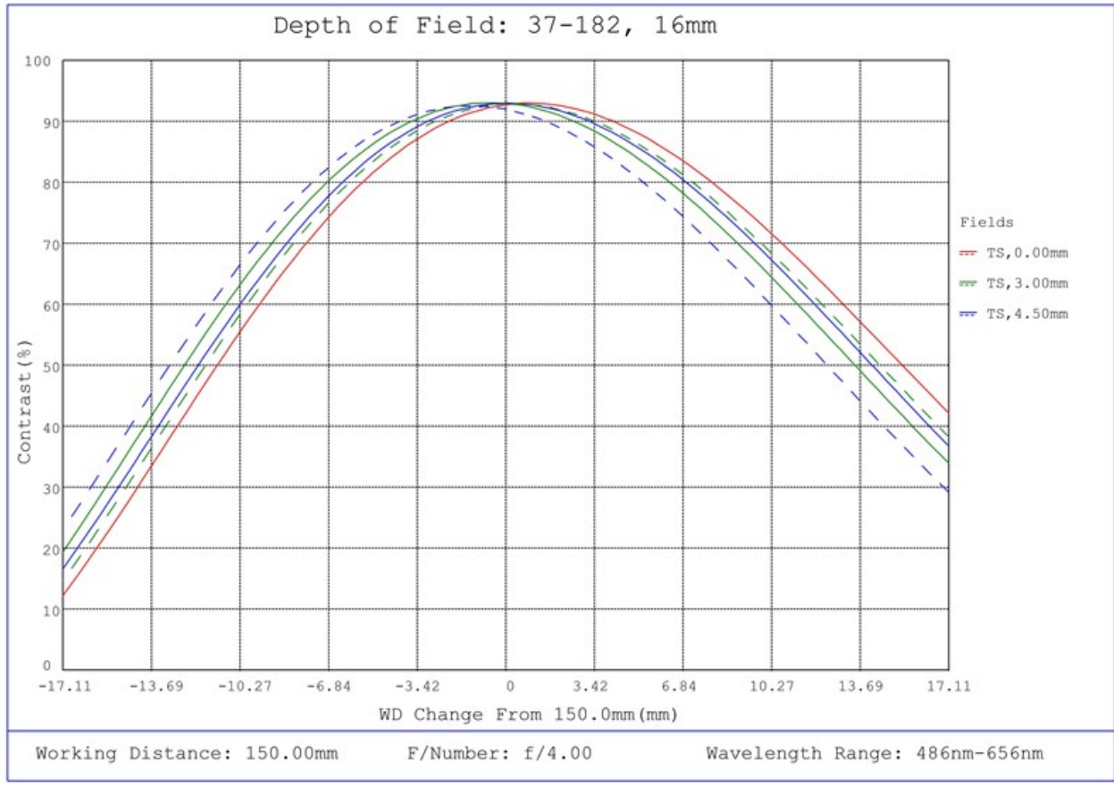
#37-182, 16mm FL f/4.0 Blue Series M12 Lens, Depth of Field Plot, 150mm Working Distance, f4
