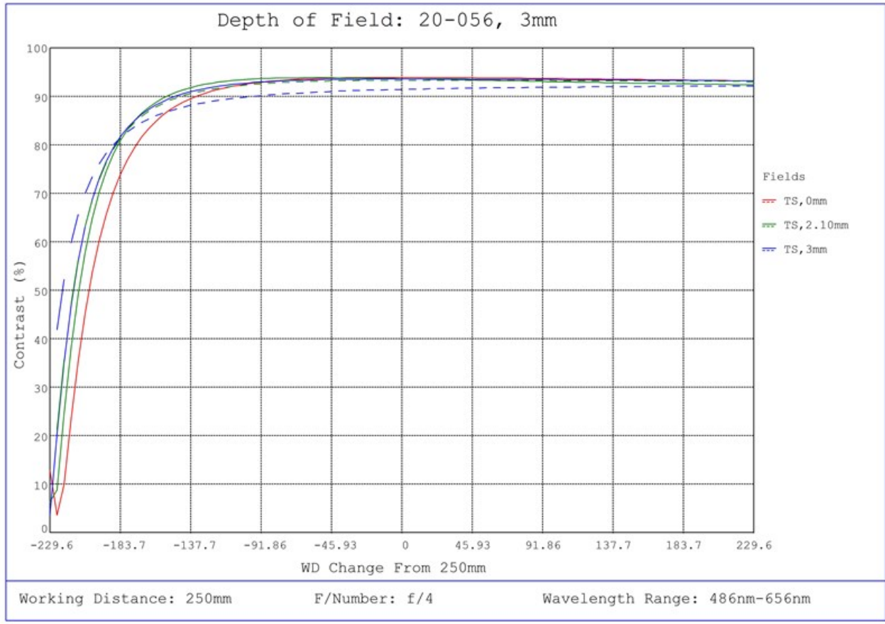
#20-056, 3mm FL f/4.0, IR-Cut Blue Series M12 Lens, Depth of Field Plot, 250mm Working Distance, f4
