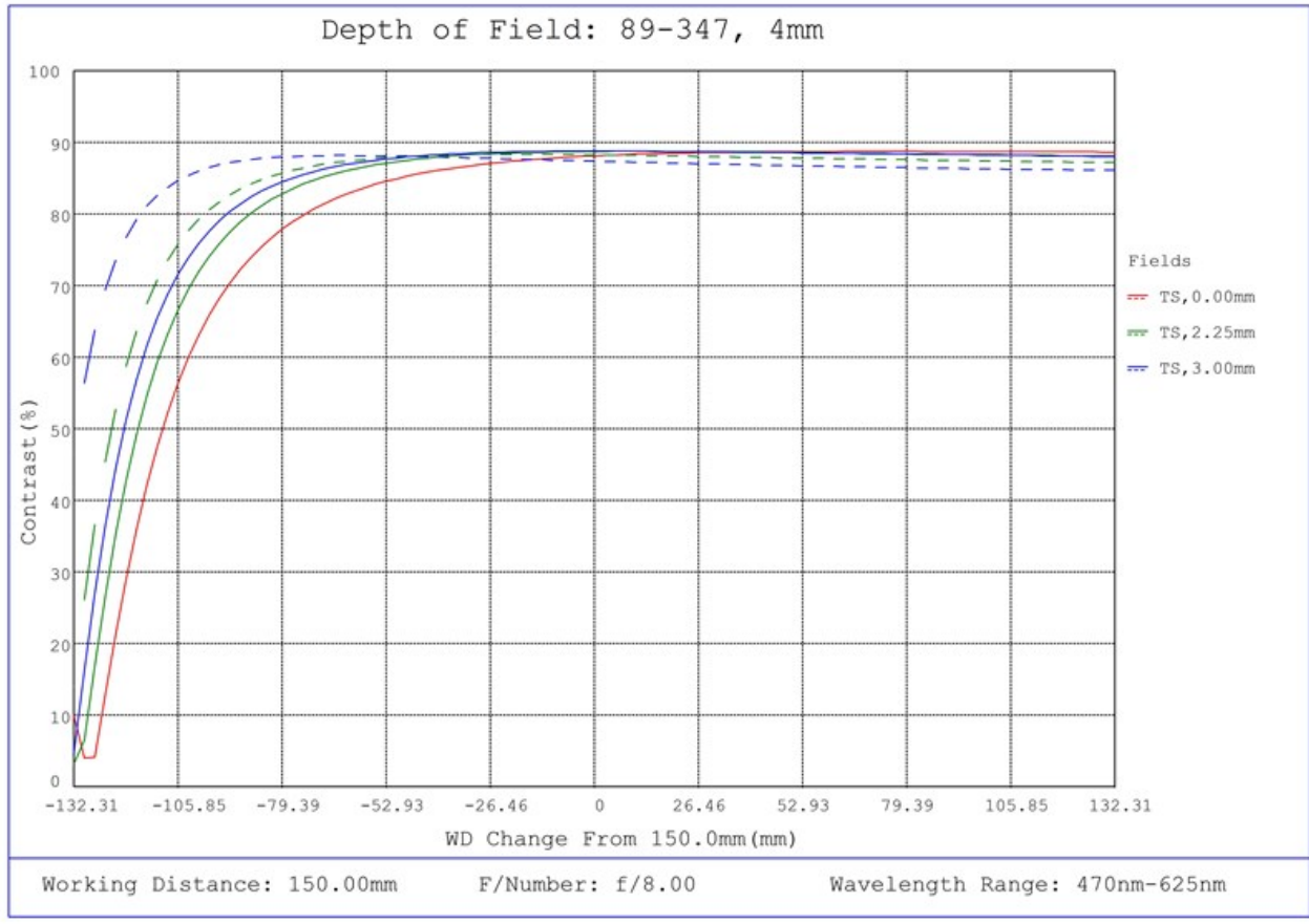
#89-347, 4mm FL f/8.0, Blue Series M12 Lens, Depth of Field Plot, 150mm Working Distance, f8
