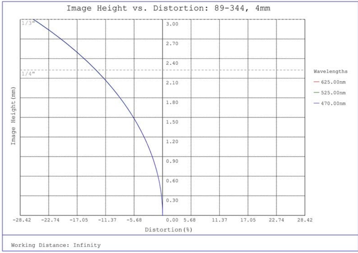
#89-344, 4mm FL f/2.5, Blue Series M12 Lens, Distortion Plot
