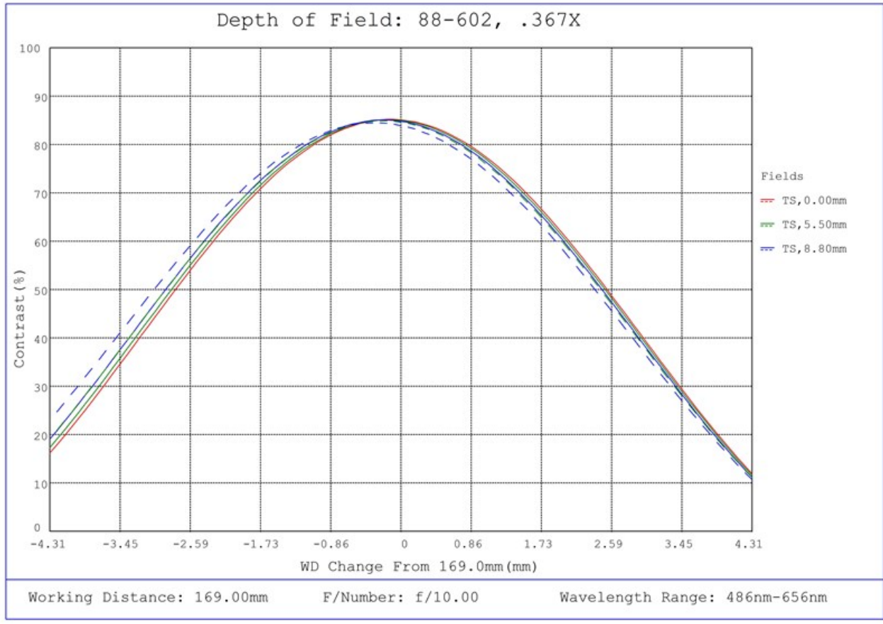
#88-602, 0.367X CobaltTL Telecentric Lens, Depth of Field Plot, 169mm Working Distance, f10
