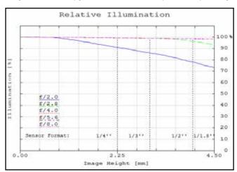
Figure 2: Relative illumination (center to corner)
