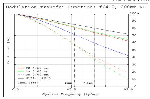
Figure 5: Image space polychromatic diffraction FFT Modulation Transfer Function (MTF) for λ = 486nm to 656nm. Included are Tangential and Sagittal values for field points on center, at 70% of full field and at the maximum sensor format. Solid black line indicates diffraction limit determined by f/#-defined aperture. Frequencies corresponding to the Nyquist resolution limit of pixel sizes are indicated.
