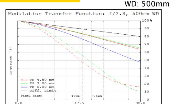
Figure 7: Image space polychromatic diffraction FFT Modulation Transfer Function (MTF) for  $\lambda = 486$ nm to 656nm. Included are Tangential and Sagittal values for field points on center, at 70% of full field and at the maximum sensor format. Solid black line indicates diffraction limit determined by f/#-defined aperture. Frequencies corresponding to the Nyquist resolution limit of pixel sizes are indicated.
