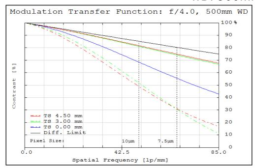
Figure 9: Image space polychromatic diffraction FFT Modulation Transfer Function (MTF) for λ = 486nm to 656nm. Included are Tangential and Sagittal values for field points on center, at 70% of full field and at the maximum sensor format. Solid black line indicates diffraction limit determined by f/#-defined aperture. Frequencies corresponding to the Nyquist resolution limit of pixel sizes are indicated.
