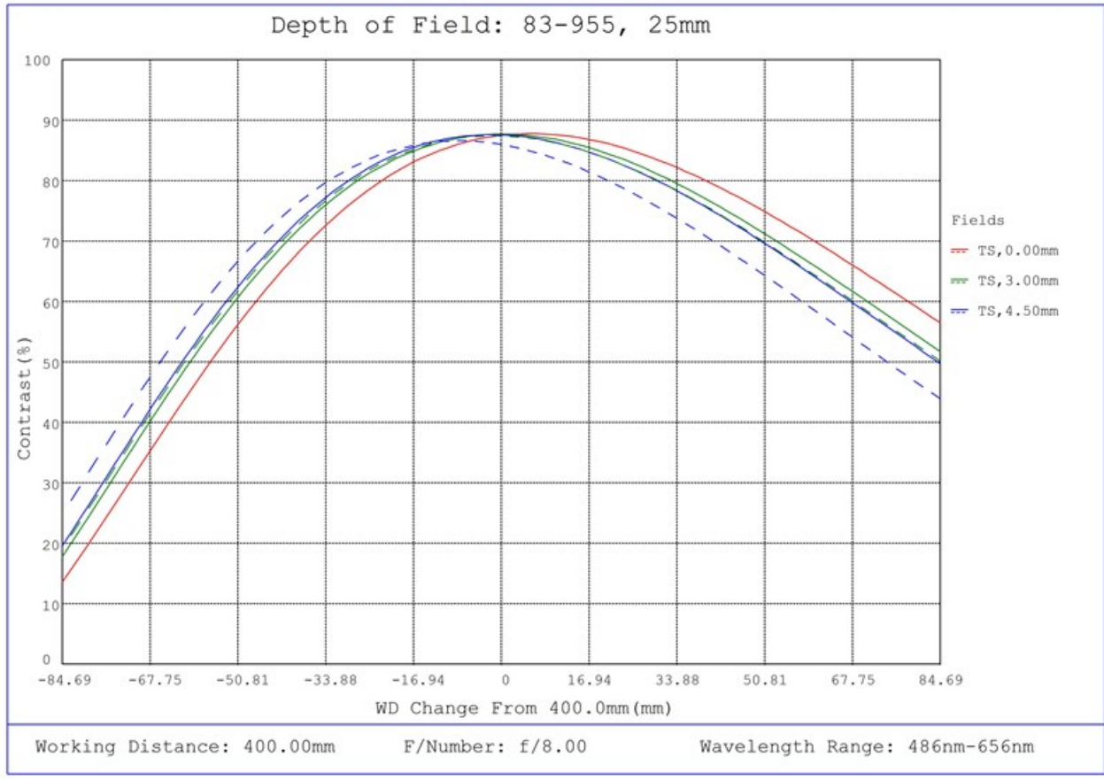
#83-955, 25mm FL f/8, Blue Series M12 Lens, Depth of Field Plot, 400mm Working Distance, f8
