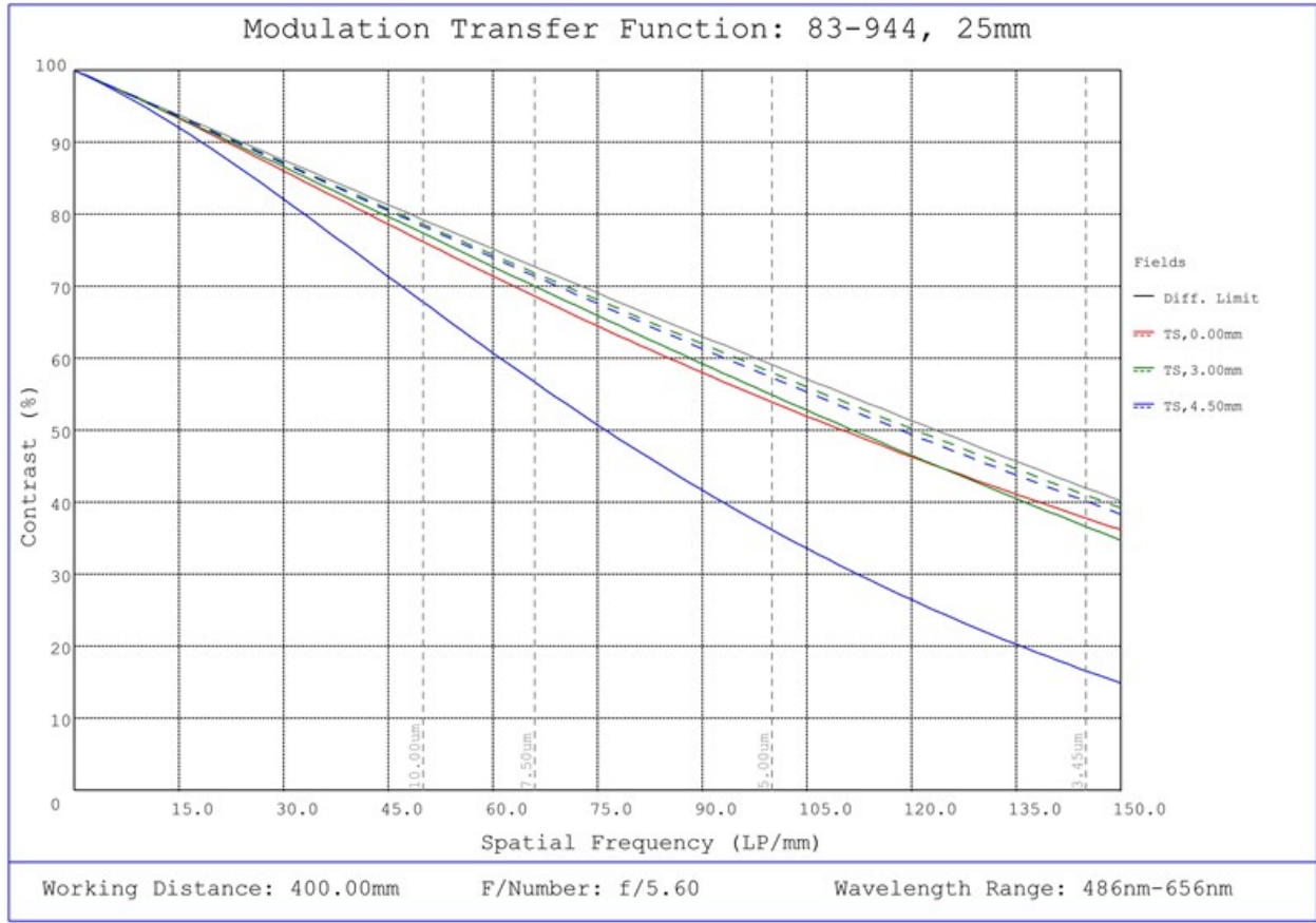
#83-944, 25mm FL f/5.6, Blue Series M12 Lens, Modulated Transfer Function (MTF) Plot, 400mm Working Distance, f5.6
