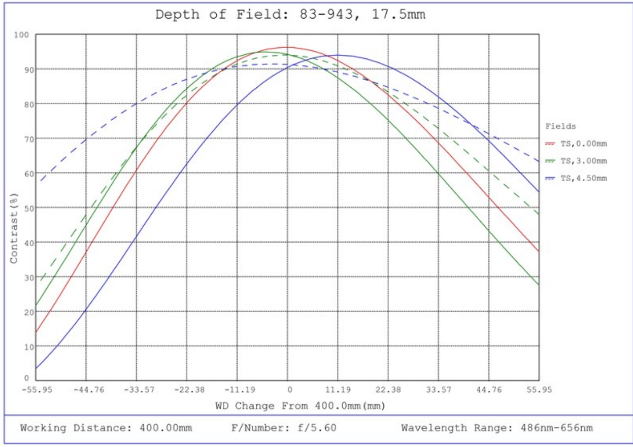
#83-943, 17.5mm FL f/5.6, Blue Series M12 Lens, Depth of Field Plot, 400mm Working Distance, f5.6
