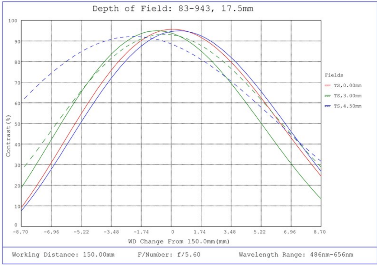
#83-943, 17.5mm FL f/5.6, Blue Series M12 Lens, Depth of Field Plot, 150mm Working Distance, f5.6
