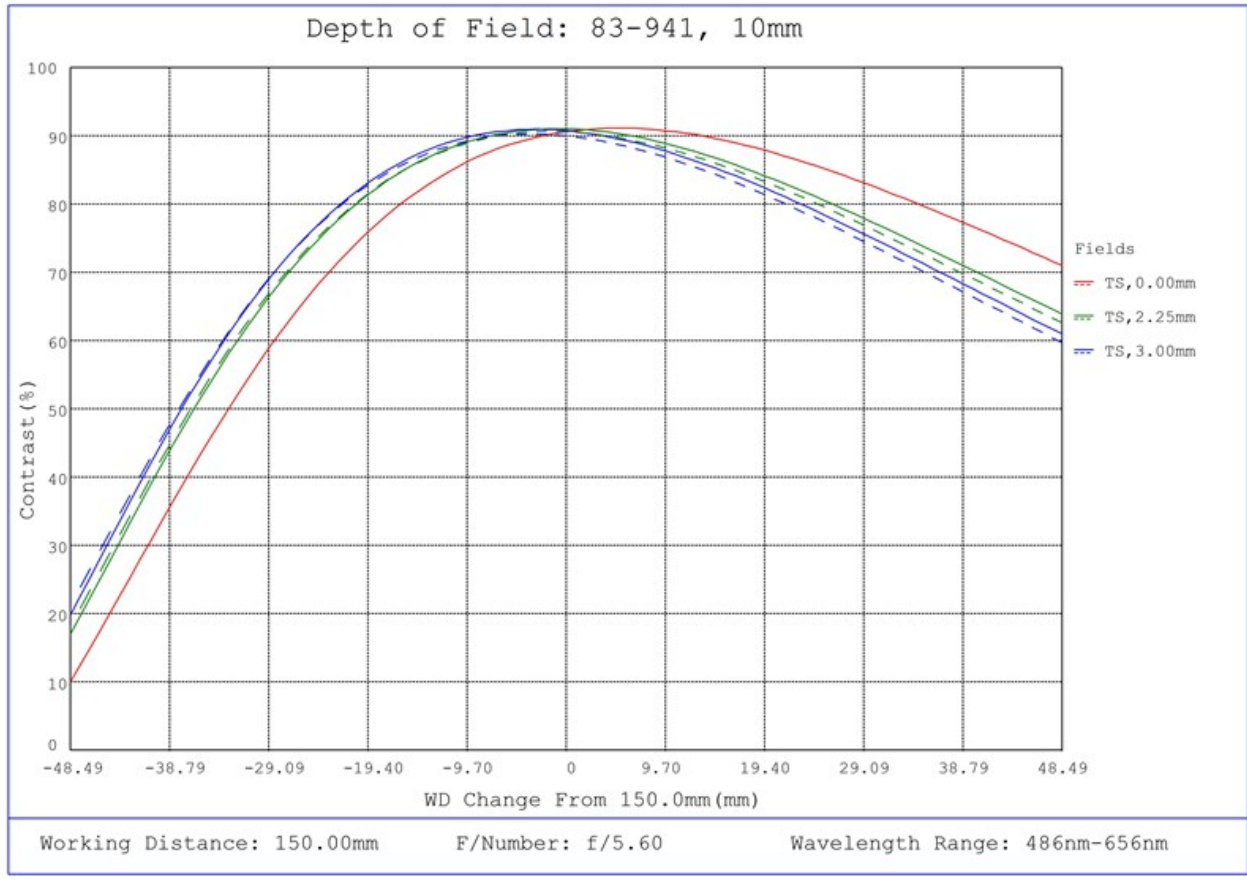
#83-941, 10mm FL f/5.6, Blue Series M12 Lens, Depth of Field Plot, 150mm Working Distance, f5.6
