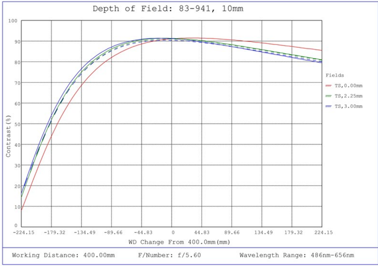
#83-941, 10mm FL f/5.6, Blue Series M12 Lens, Depth of Field Plot, 400mm Working Distance, f5.6
