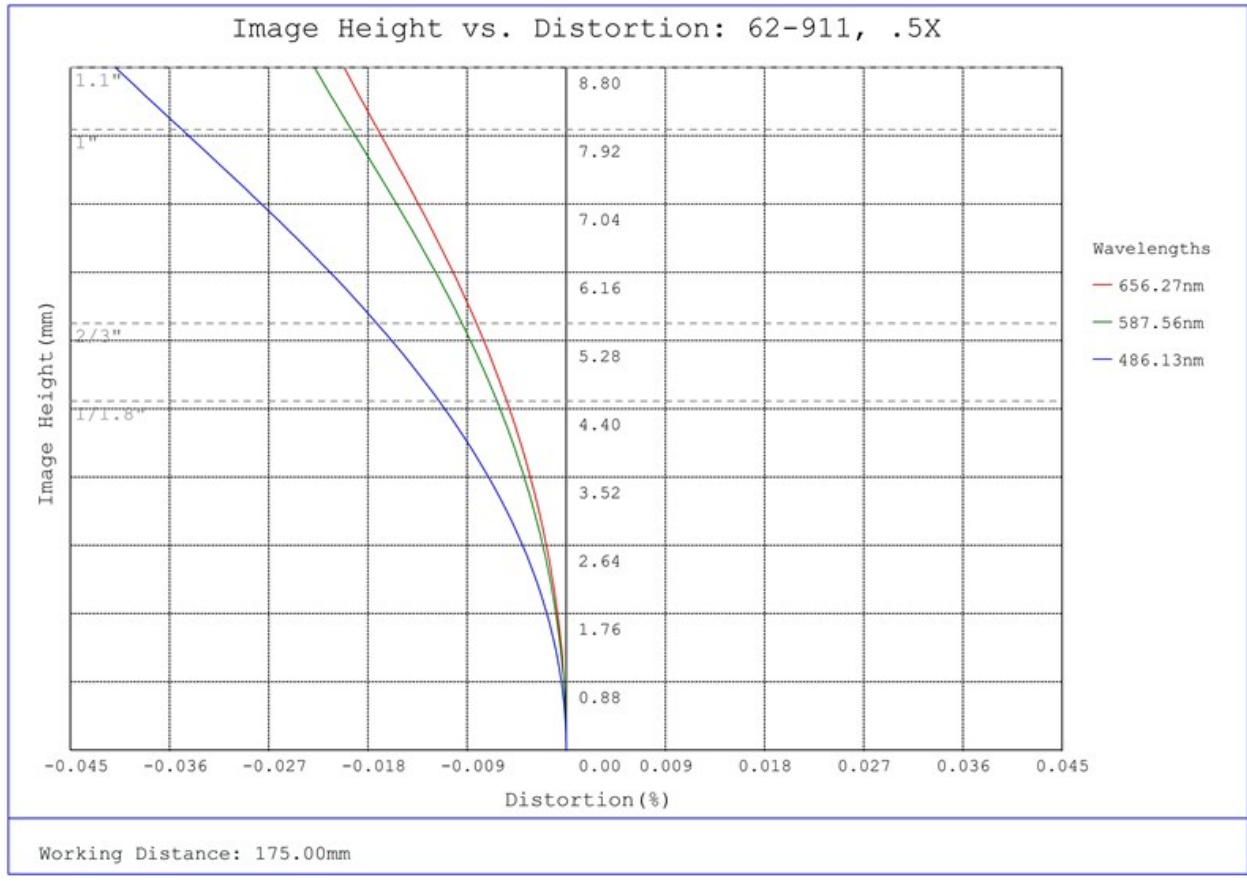
#62-911, 0.5X CobaltTL Telecentric Lens, Distortion Plot
