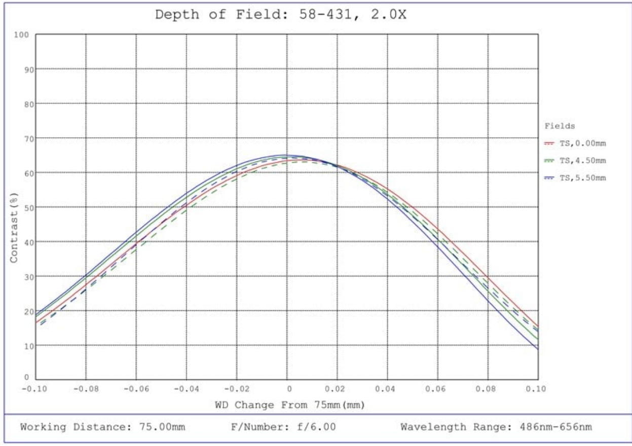
#58-431, 2.0X SilverTL™ Telecentric Lens, Depth of Field Plot, 75mm Working Distance, f6
