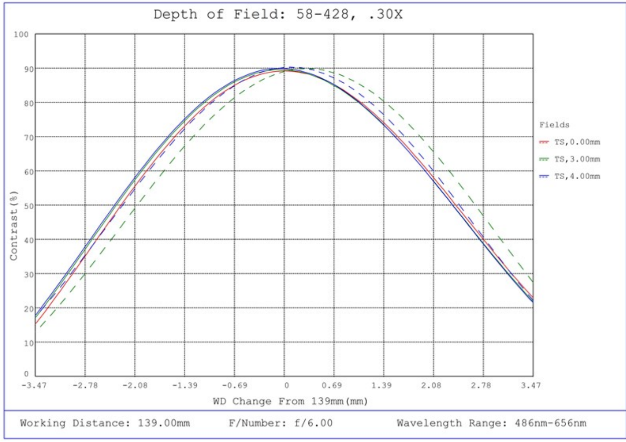
#58-428, 0.30X SilverTL™ Telecentric Lens, Depth of Field Plot, 139mm Working Distance, f6
