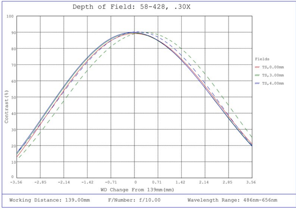
#58-428, 0.30X SilverTL™ Telecentric Lens, Depth of Field Plot, 139mm Working Distance, f10
