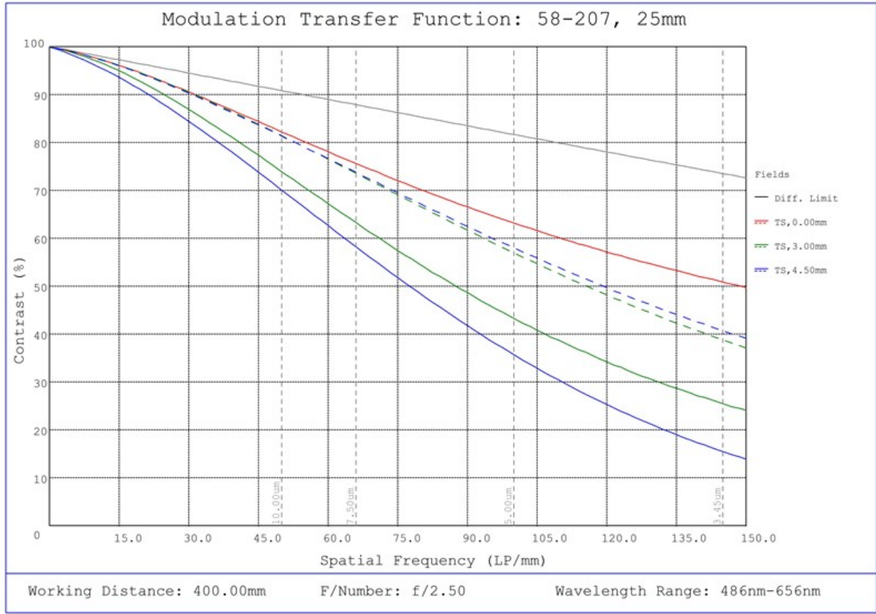
#58-207, 25mm FL f/2.5, Blue Series M12 Lens, Modulated Transfer Function (MTF) Plot, 400mm Working Distance, f2.5
