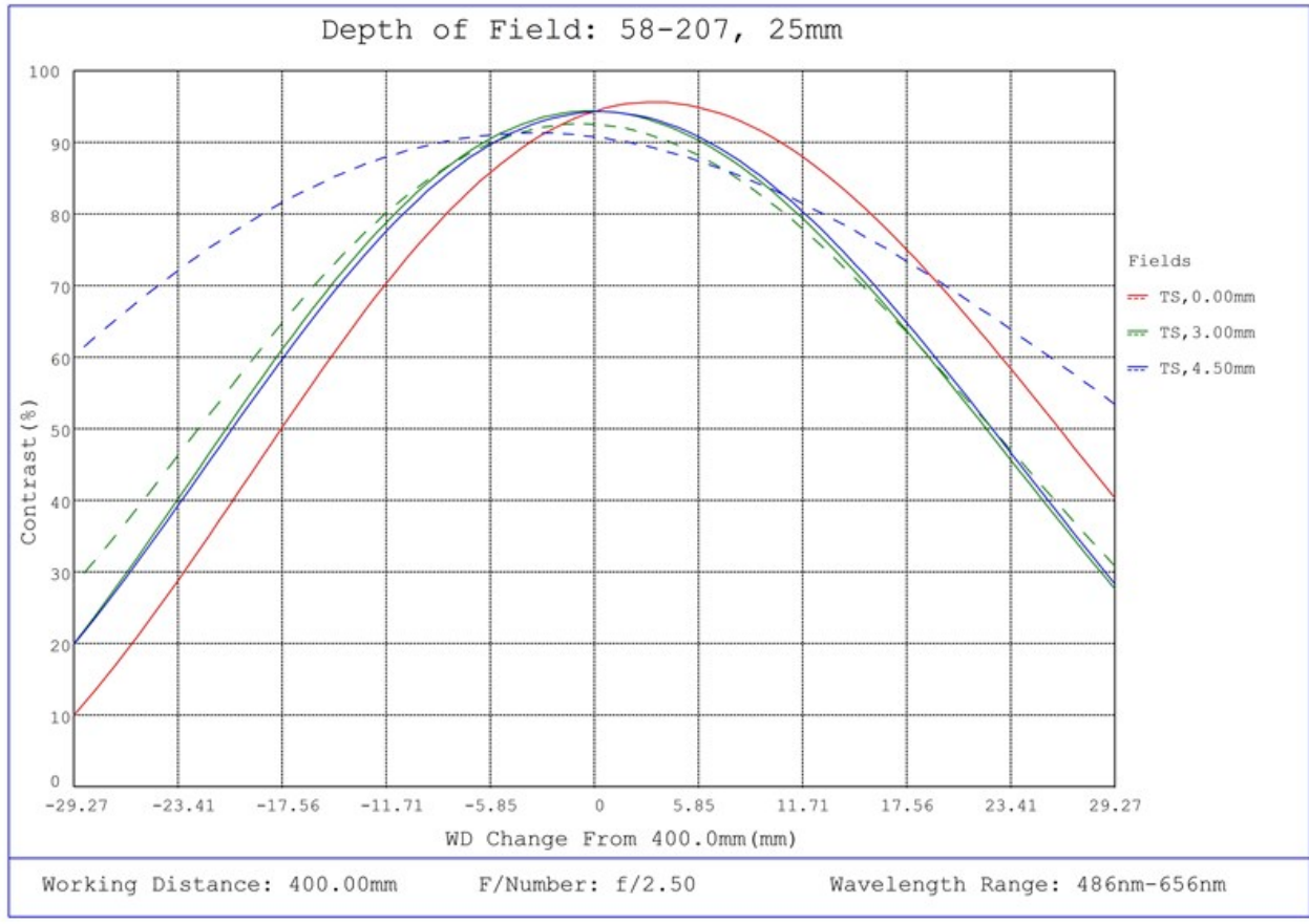
#58-207, 25mm FL f/2.5, Blue Series M12 Lens, Depth of Field Plot, 400mm Working Distance, f2.5
