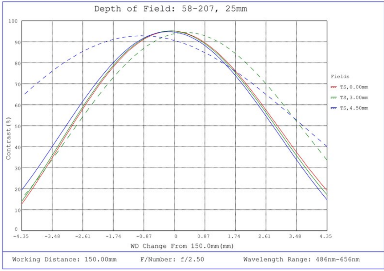
#58-207, 25mm FL f/2.5, Blue Series M12 Lens, Depth of Field Plot, 150mm Working Distance, f2.5
