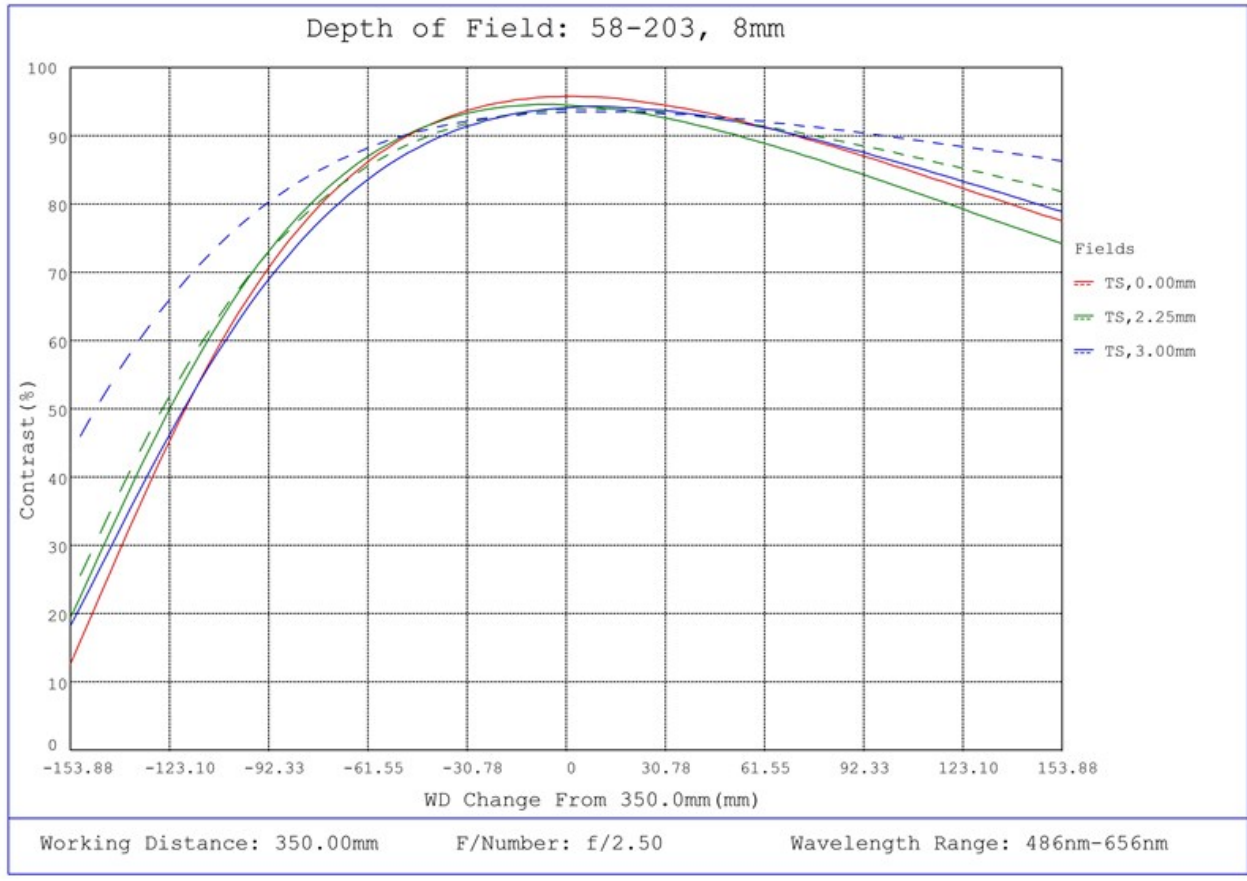
#58-203, 8mm FL f/2.5, Blue Series M12 Lens, Depth of Field Plot, 350mm Working Distance, f2.5
