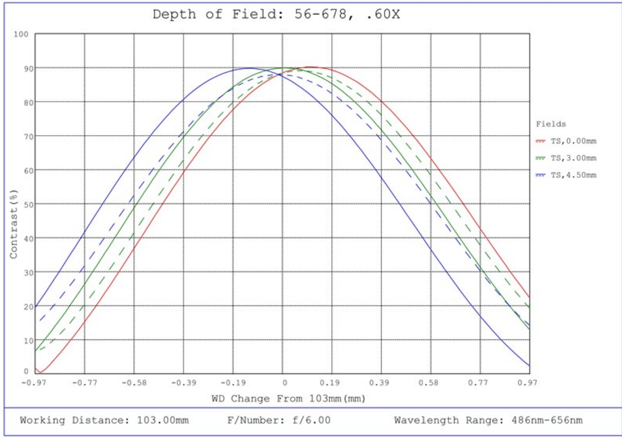
#56-678, 0.60X SilverTL™ Telecentric Lens, Depth of Field Plot, 103mm Working Distance, f6
