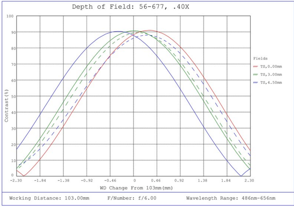
#56-677, 0.40X SilverTL™ Telecentric Lens, Depth of Field Plot, 103mm Working Distance, f6
