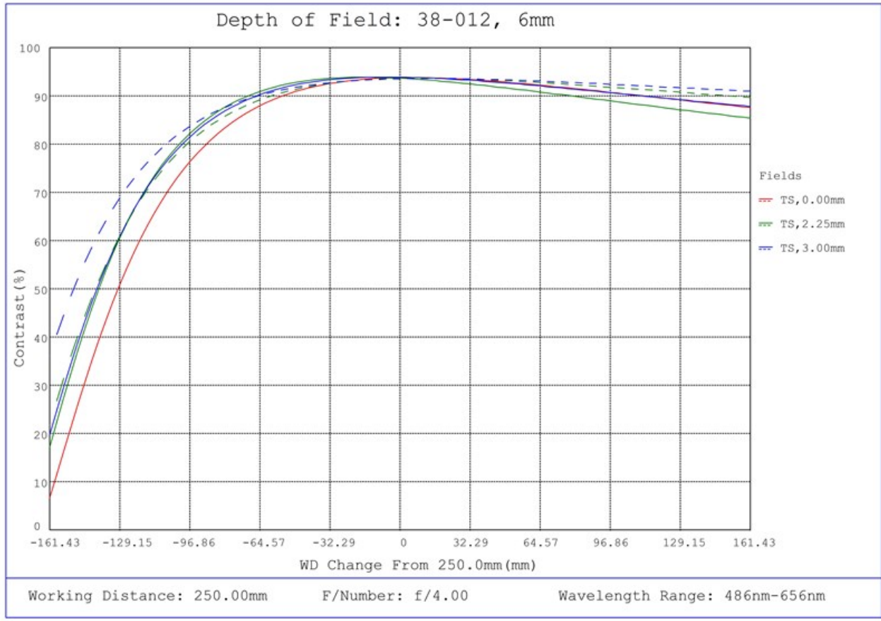
#38-012, 6mm FL f/4, Blue Series M12 Lens, Depth of Field Plot, 250mm Working Distance, f4
