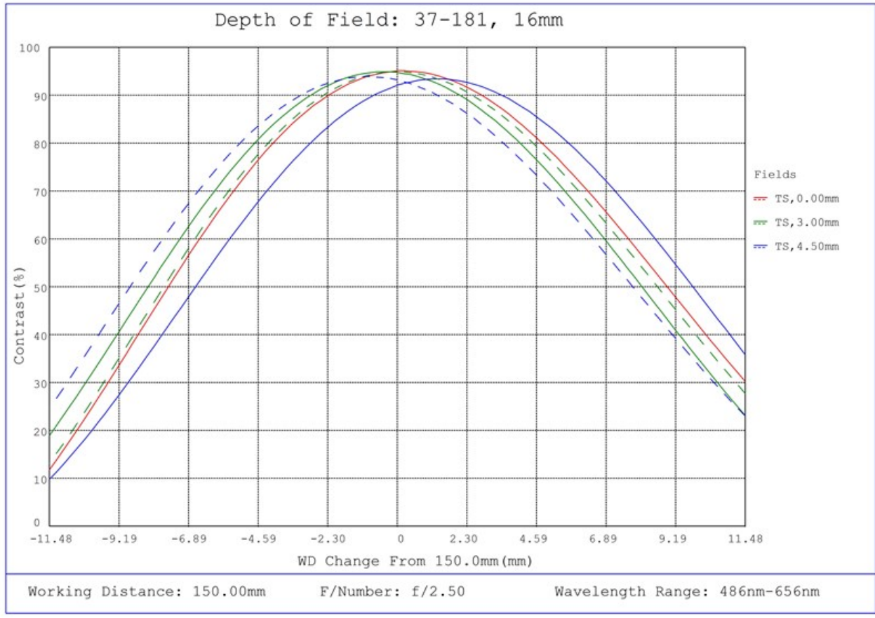
#37-181, 16mm FL f/2.5 Blue Series M12 Lens, Depth of Field Plot, 150mm Working Distance, f2.5
