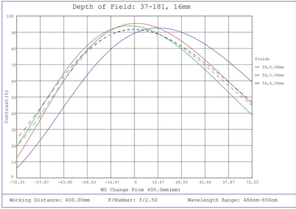
#37-181, 16mm FL f/2.5 Blue Series M12 Lens, Depth of Field Plot, 400mm Working Distance, f2.5
