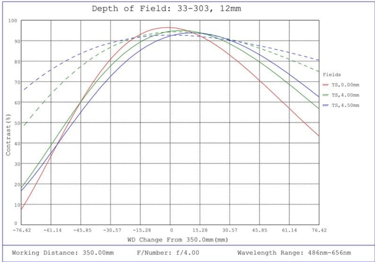
#33-303, 12mm UC Series Fixed Focal Length Lens, Depth of Field Plot, 350mm Working Distance, f4
