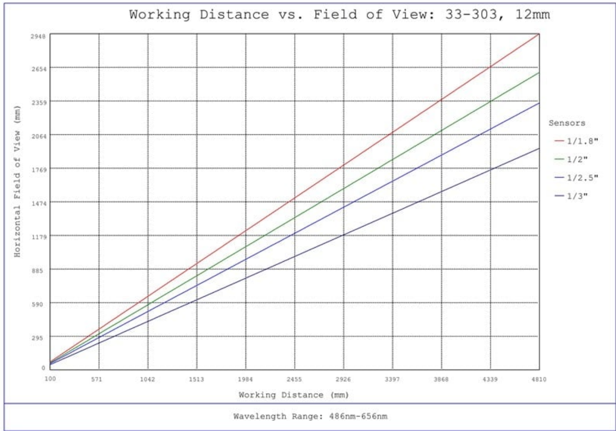
#33-303, 12mm UC Series Fixed Focal Length Lens, Working Distance versus Field of View Plot
