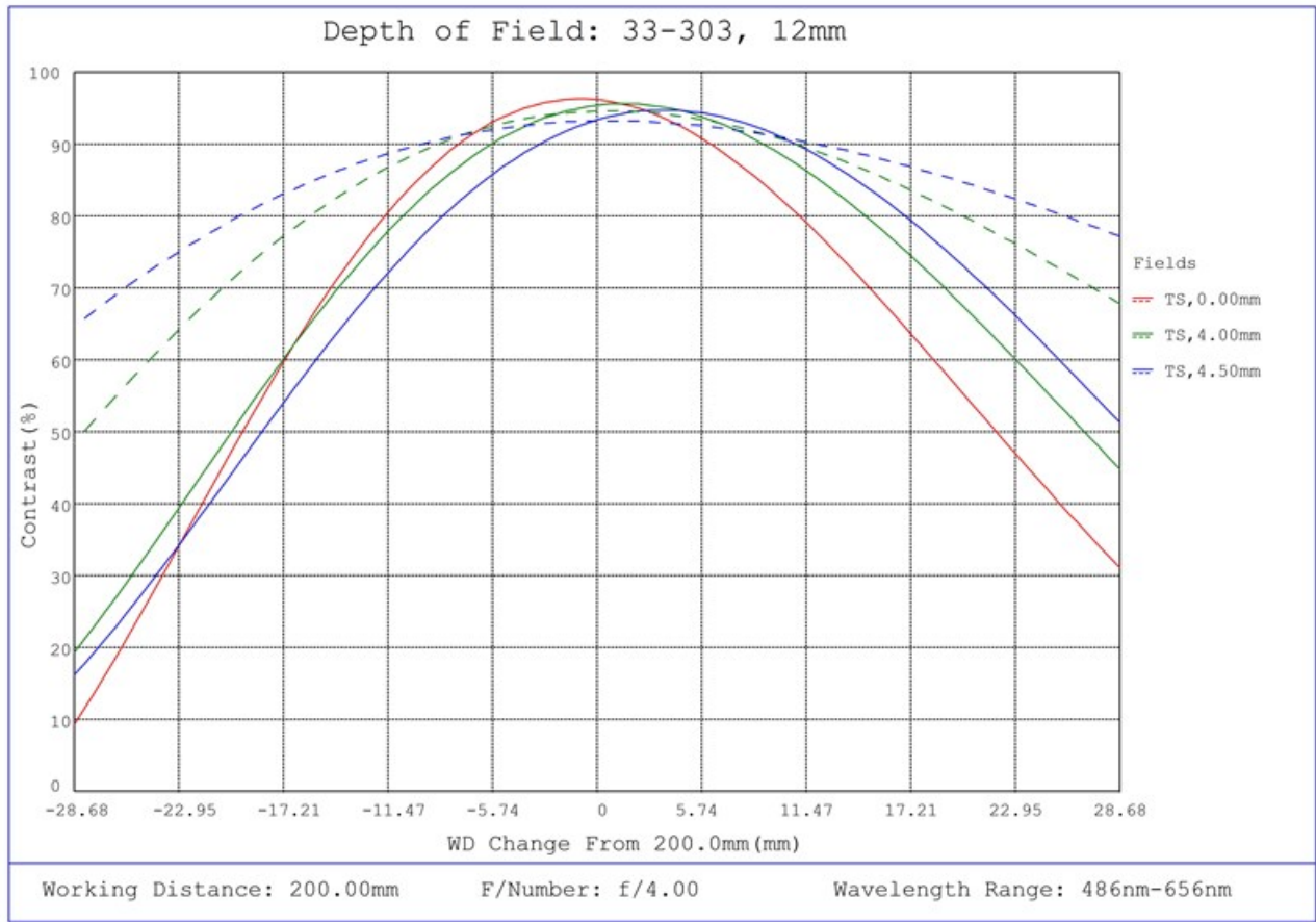
#33-303, 12mm UC Series Fixed Focal Length Lens, Depth of Field Plot, 200mm Working Distance, f4
