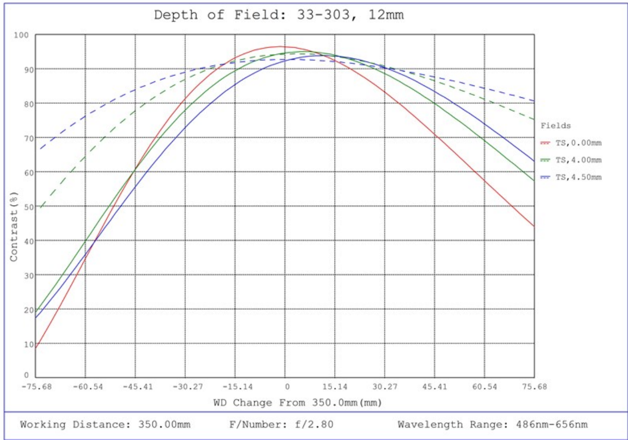
#33-303, 12mm UC Series Fixed Focal Length Lens, Depth of Field Plot, 350mm Working Distance, f2.8
