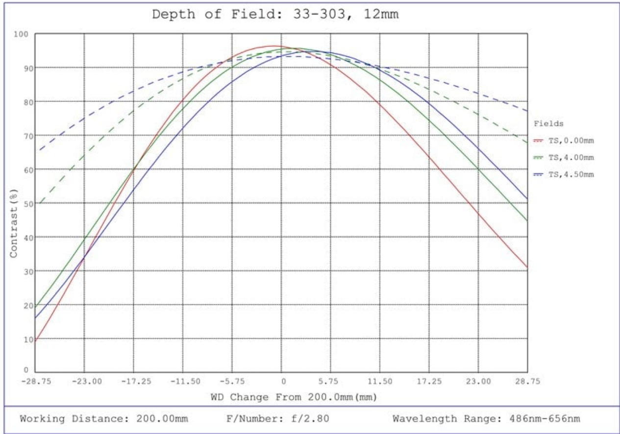
#33-303, 12mm UC Series Fixed Focal Length Lens, Depth of Field Plot, 200mm Working Distance, f2.8
