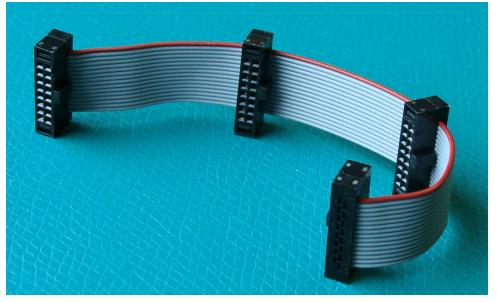
Figure 39: Photo of cable OR-YXCC-BSYNC40
