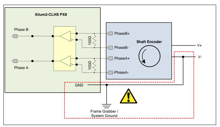
Figure 31: RS-422 Shaft Encoder Input Electrical Diagram
