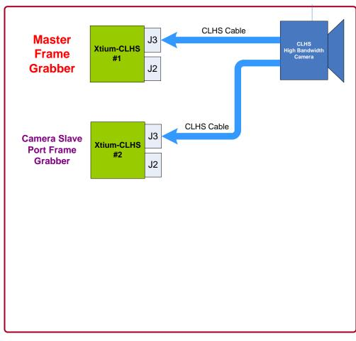
Figure 25: Dual Camera Output Connection Block Diagram
