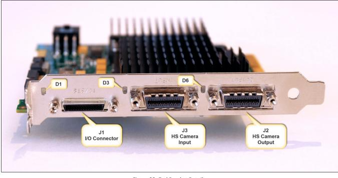
Figure 23: End Bracket Details
