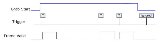
Figure 17: Line scan, Fixed Frame, Edge Trigger
