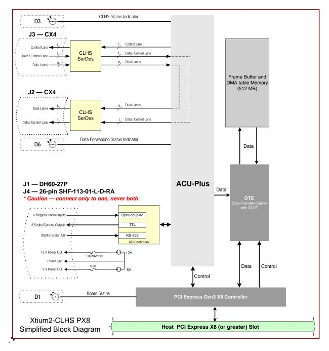
Figure 10: Xtium2-CLHS PX8 Block Diagram
