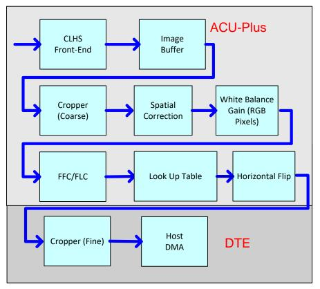
Figure 11: Xtium2-CLHS Flow Diagram
