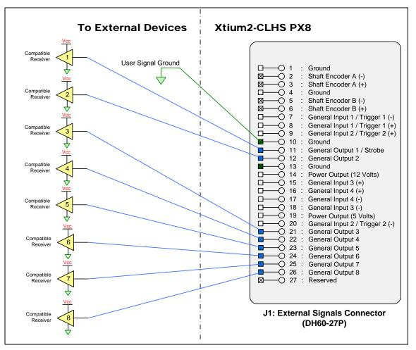
Figure 30:Output Signals Connection Diagram
