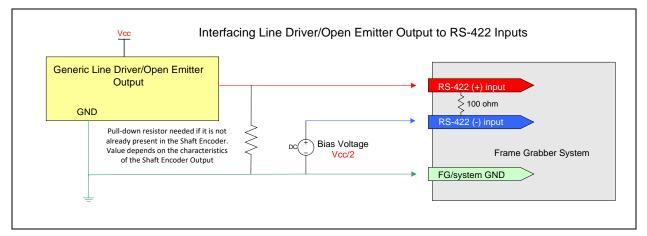
Figure 34: Interfacing to a Line Driver Output
