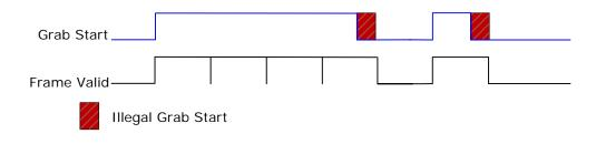
Figure 16: Line scan, Fixed Frame, No Trigger
