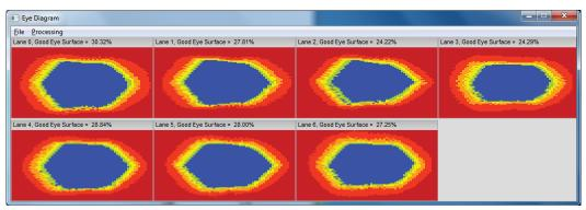
Figure 44: Diagnostic Tool Eye Diagram
