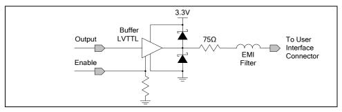
Figure 29: General Outputs Electrical Diagram
