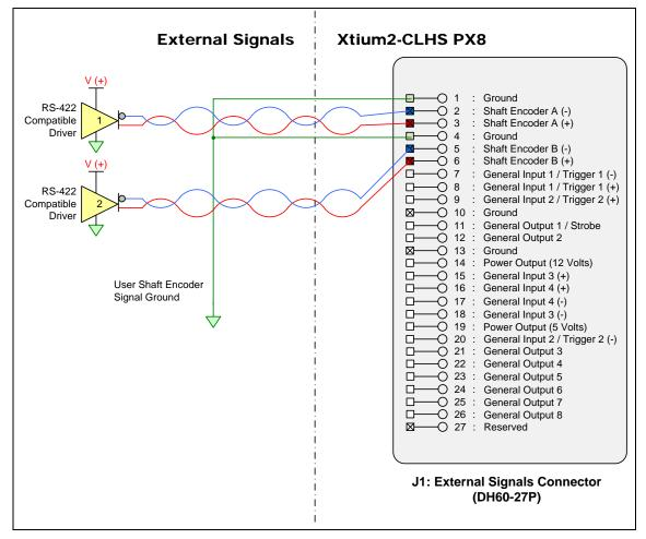
Figure 32:External RS-422 Signals Connection Diagram
