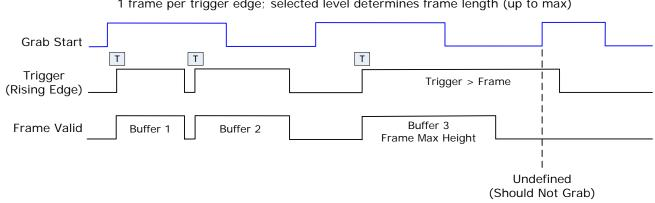
1 frame per trigger edge; selected level determines frame length (up to max)
