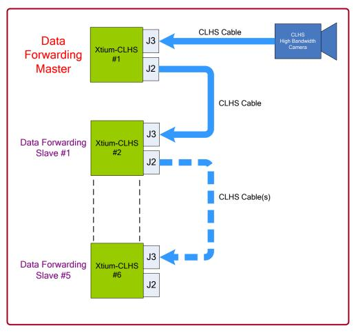
Figure 24: Data Forwarding Block Diagram
