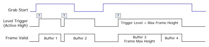
Figure 20: Line scan, Fixed Frame, Level Trigger (Roll-Over)
