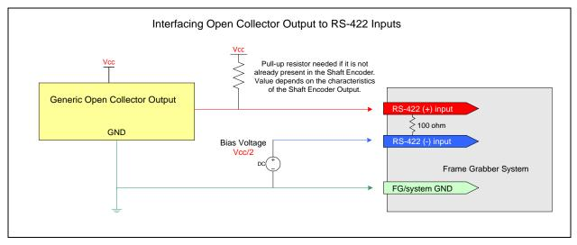
Figure 35: Interfacing to an Open Collector Output
