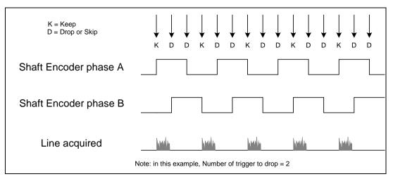
Figure 13: Encoder Input with Pulse-drop Counter
