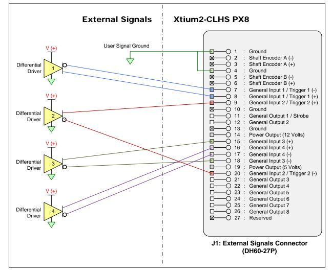
Block Diagram: Connecting External Drivers to General Inputs on J1
