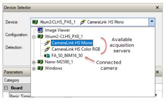
The Xtium2-CLHS PX8 firmware supports one Camera Link HS camera and provides the following acquisition servers:
