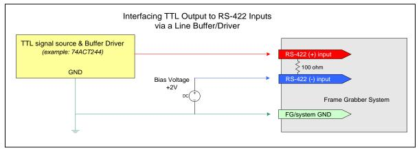
Figure 33: Interfacing TTL to RS-422 Shaft Encoder Inputs
