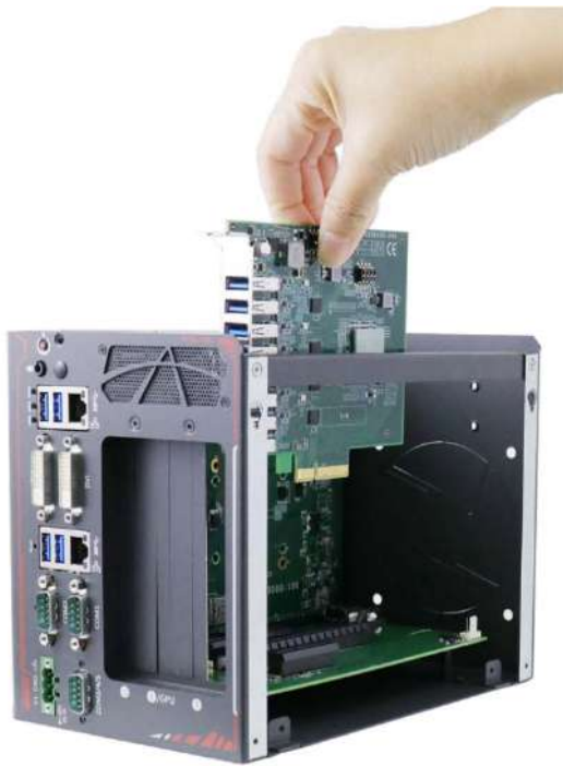
Lower PCIe-USB381F into the case
