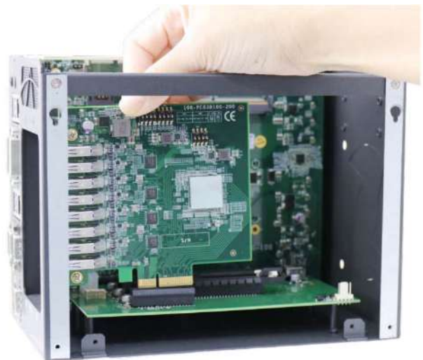
Insert gold finger into PCIe slot
