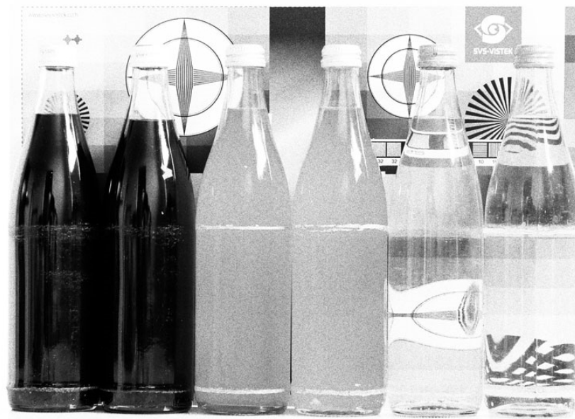
Fig.: 6-3: Noise caused by too much gain
