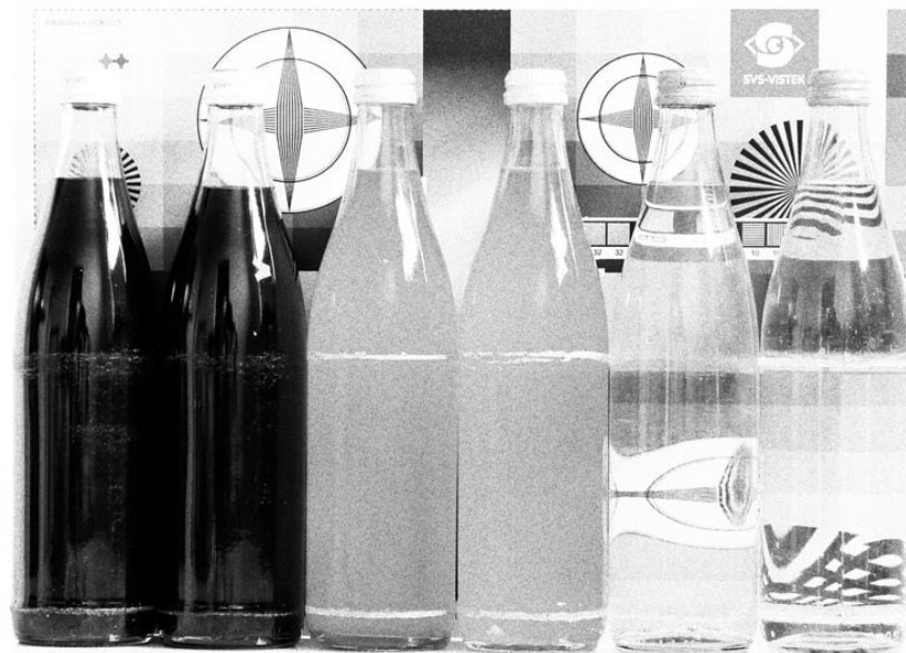
Fig.: 6-1: Noise caused by too much gain
