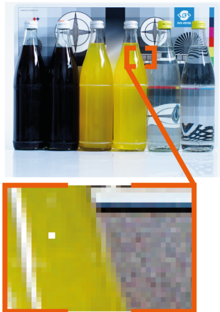
Fig.: 6-24: Illustration of a defect pixel
