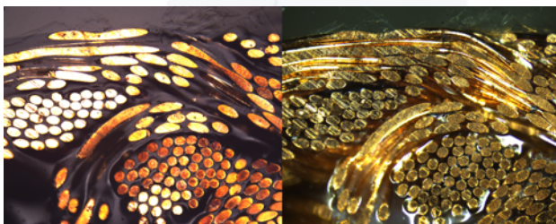
Fig.7: Colour crimp images - IM · bright field (left) vs. IM · dark field (right)
