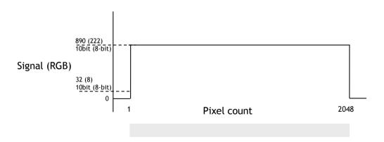
Fig. 19 White level test pattern
