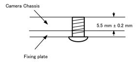
Fixing the camera on the plate
