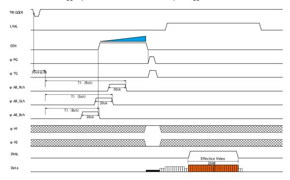
Fig. 15 Shutter-Select mode with external trigger (and individual exposure)
