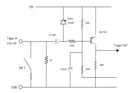
Fig. 6 Trigger input (12-pin Hirose)
