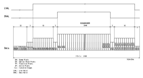
Fig.11 Video output timing
