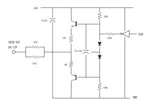
Fig. 7 XEEN Circuit (12-pin Hirose)
