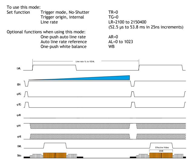
Fig. 12 No-Shutter mode with internal line rate generator
