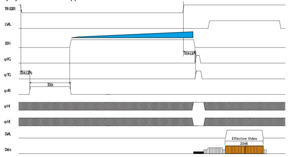
Fig. 16 Pulse Width Control mode
