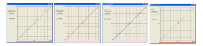
When you drag the line and move it, the required gamma characteristics can be obtained.
