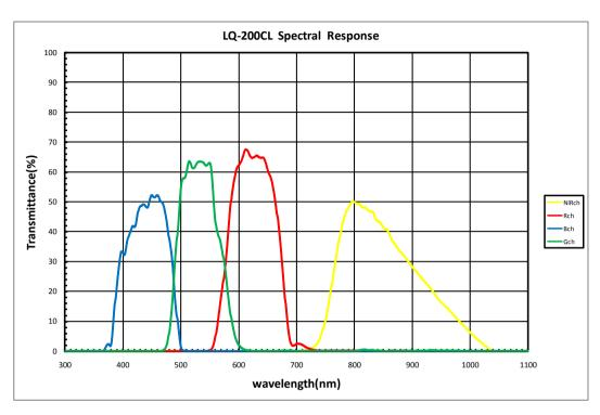
Fig. 27 Camera Spectral sensitivity
