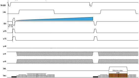
Fig. 13 No-Shutter mode with external trigger
