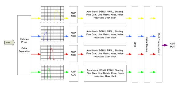
Fig.9 Signals flow
