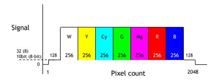
Fig. 16 Color bar test pattern
