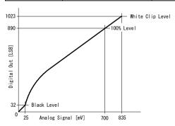
Fig. 18 LUT characteristics
