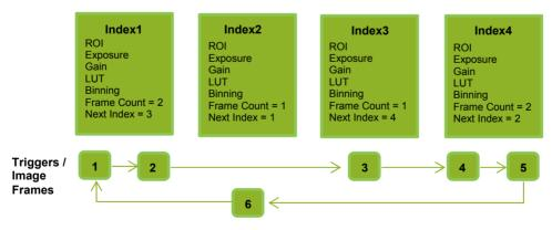
Specify "1" in [SequencerSetStart], and start TriggerSequencer mode with index 1.
