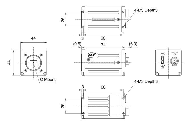
Dimensional tolerance: ±0.3 mm Unit: mm
