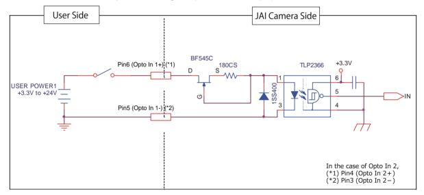
Recommended external input circuit diagram (reference example)
